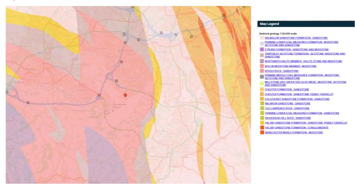
Details of the site hydrogeology were sourced from the MAGIC mapping service. The Aquifer Designation Maps show that the site is situated within a Secondary B bedrock aquifer, described as low a permeability unit that stores and yields limited amounts of groundwater through characteristics like fissures and openings or eroded layers.
