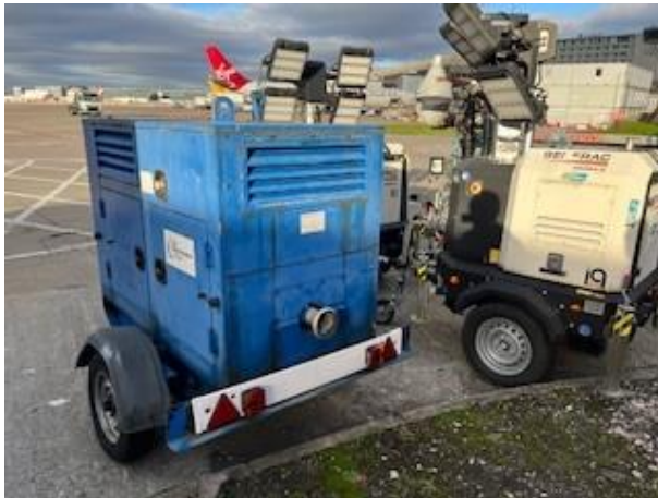
Figure 57: Mobile generator (approx. 1MWth)
