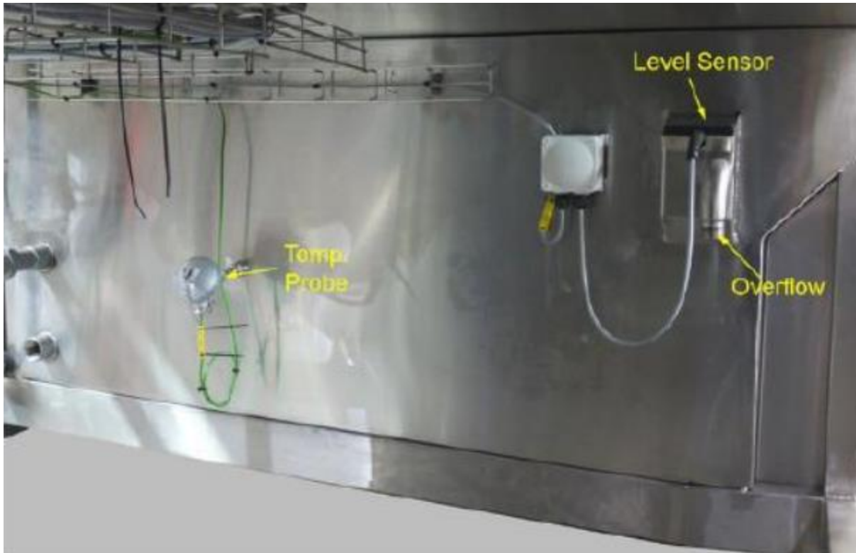
Figure 5 – Washer: Main Wash Level Probe / Overflow
