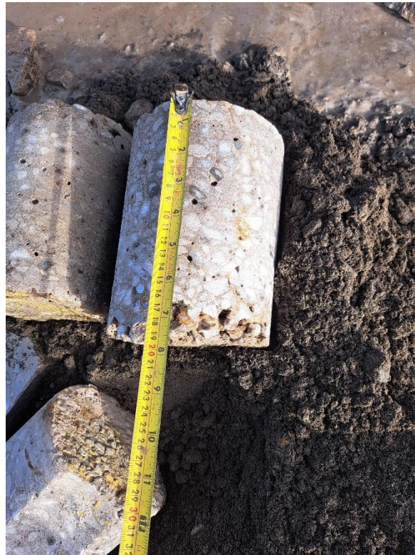
Photograph 1 BH02 inspection pit arisings and concrete core detail.
