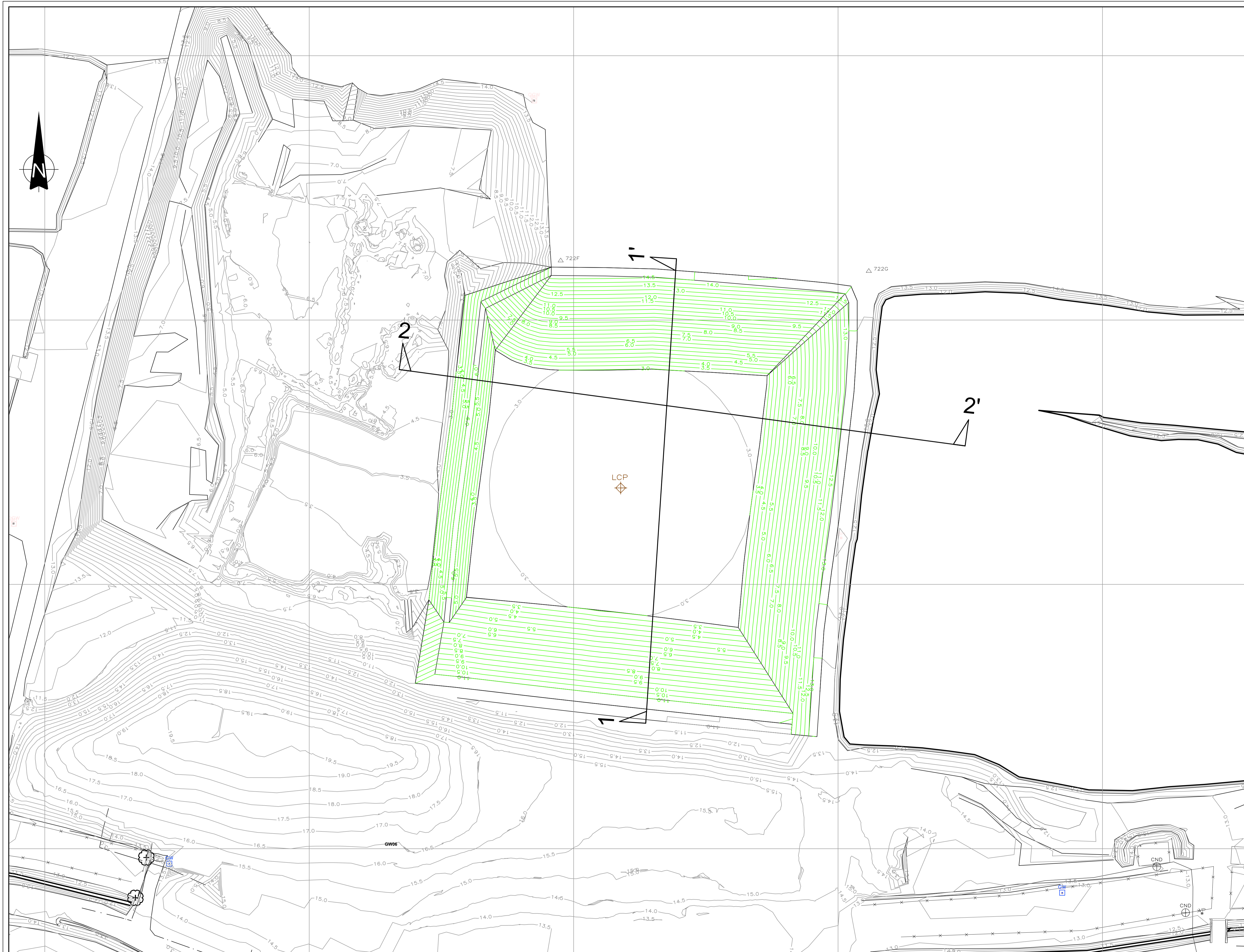
LAYOUT SHOWING PROPOSED TOP OF LINER WITH STABILITY SECTION LOCATIONS
