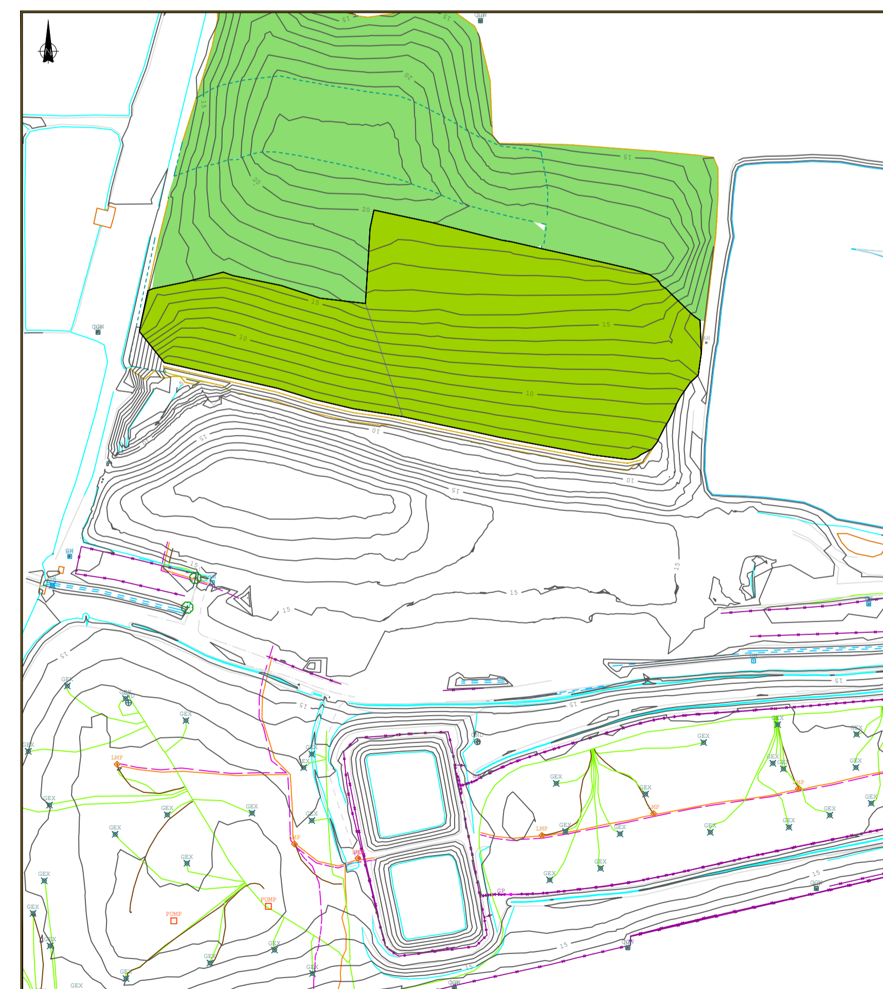
PROPOSED CELL 1, 2, 3 & 4 RESTORED - IBA PAD FILLED SCALE 1:1250
