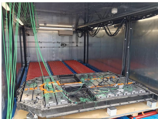
Figure 5-3 Example of Battery Discharge System
