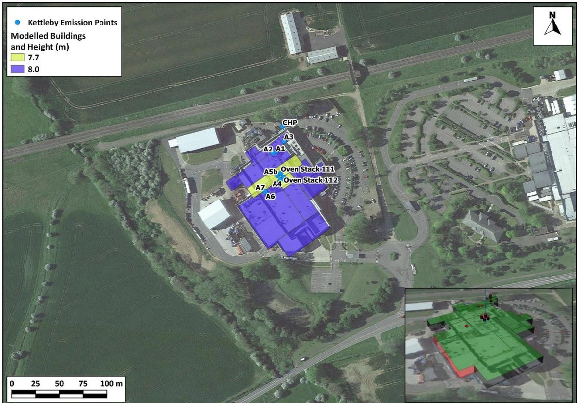
**Figure A1.2: Kettleby Buildings Included in the Model. Inset Shows 3D Image.**
