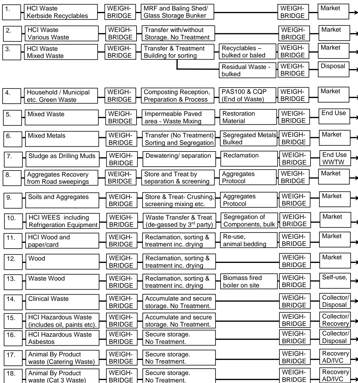
Fig. 5c- 2 Waste Flows Schematic, showing the pathways of the wastes through the Sinkfall site.
