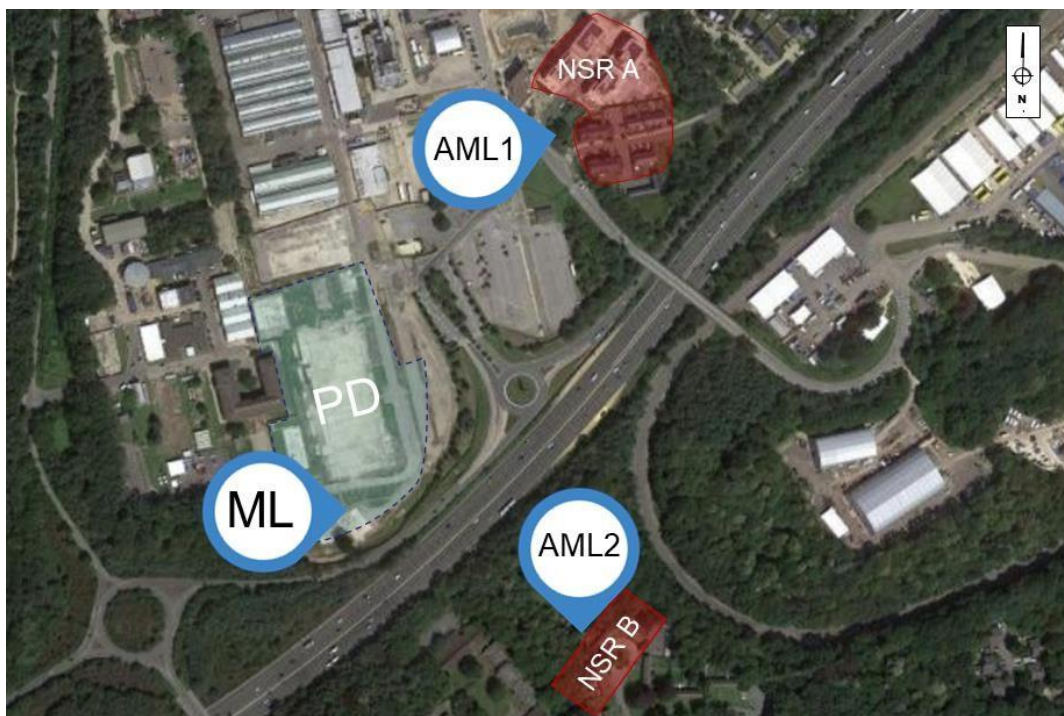
Figure 3: Noise sensitive receptors (NSRs), attended measurement locations (AMLs), long term measurement location (ML) and proposed development location (PD).
