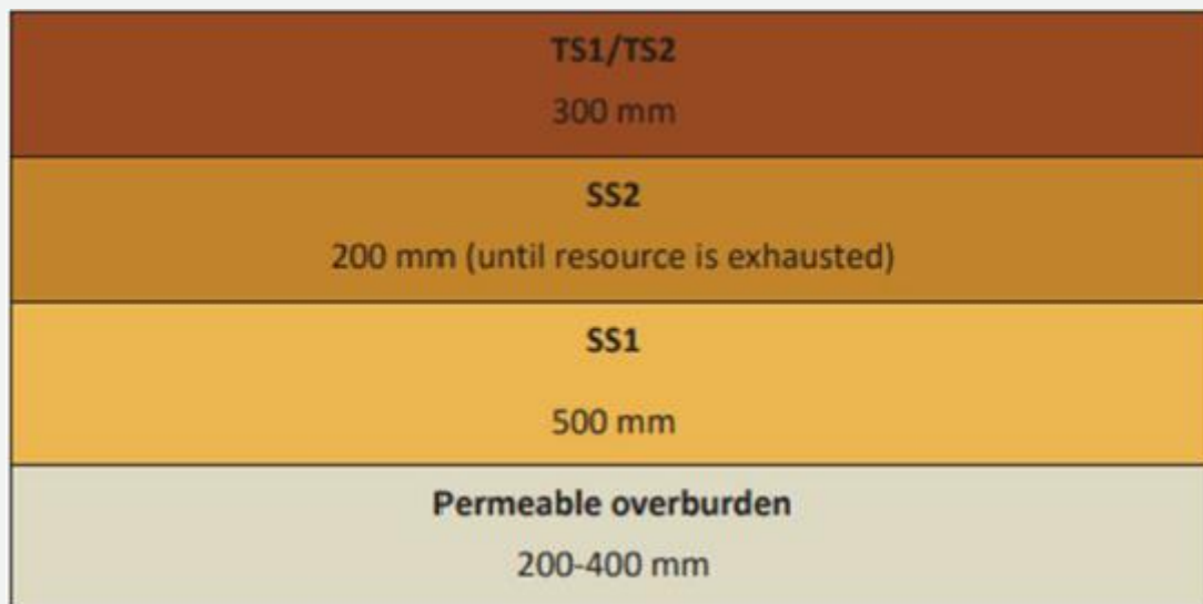
Figure 4-1: Recommended restoration soil profile to 1.2m
