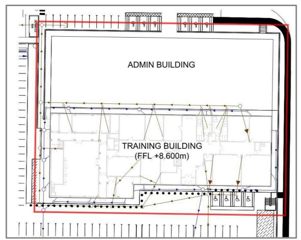
7.3.13 The 5 mm interception storage required to comply with good SuDS practice for the 2 ha Coronation Wood development area is calculated to be 100 m³. This can be adequately intercepted and captured within the infiltration systems provided for this development.
