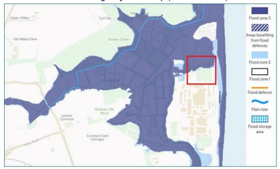
Where the site is within Flood Zone 3, flood resilience measures are required, and the design of the development will keep water out as much as possible. The platform drainage on the MCA has taken this into consideration. The WMZs also provide compensatory areas into which exceedance events may flow in a controlled manner. Drainage features will be located outside of fluvial floodplains where the design allows.
