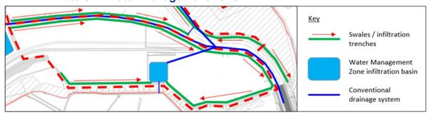
3.3.19 WMZ-2 includes contractor compounds with the main access road to the north and contains the railhead in the centre of the catchment. The drainage in this catchment includes road edge swale to the south of the main access
