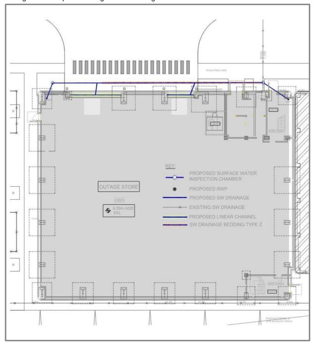
Figure 6.1 Proposed Outage Store Drainage Schematic
