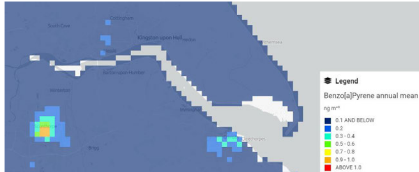
Figure 13 Maximum Annual Average Process Contribution for B[a]P ( \text{ng m}^{-3} ) with all Plant Operating Concurrently; 2019 Meteorological Data
