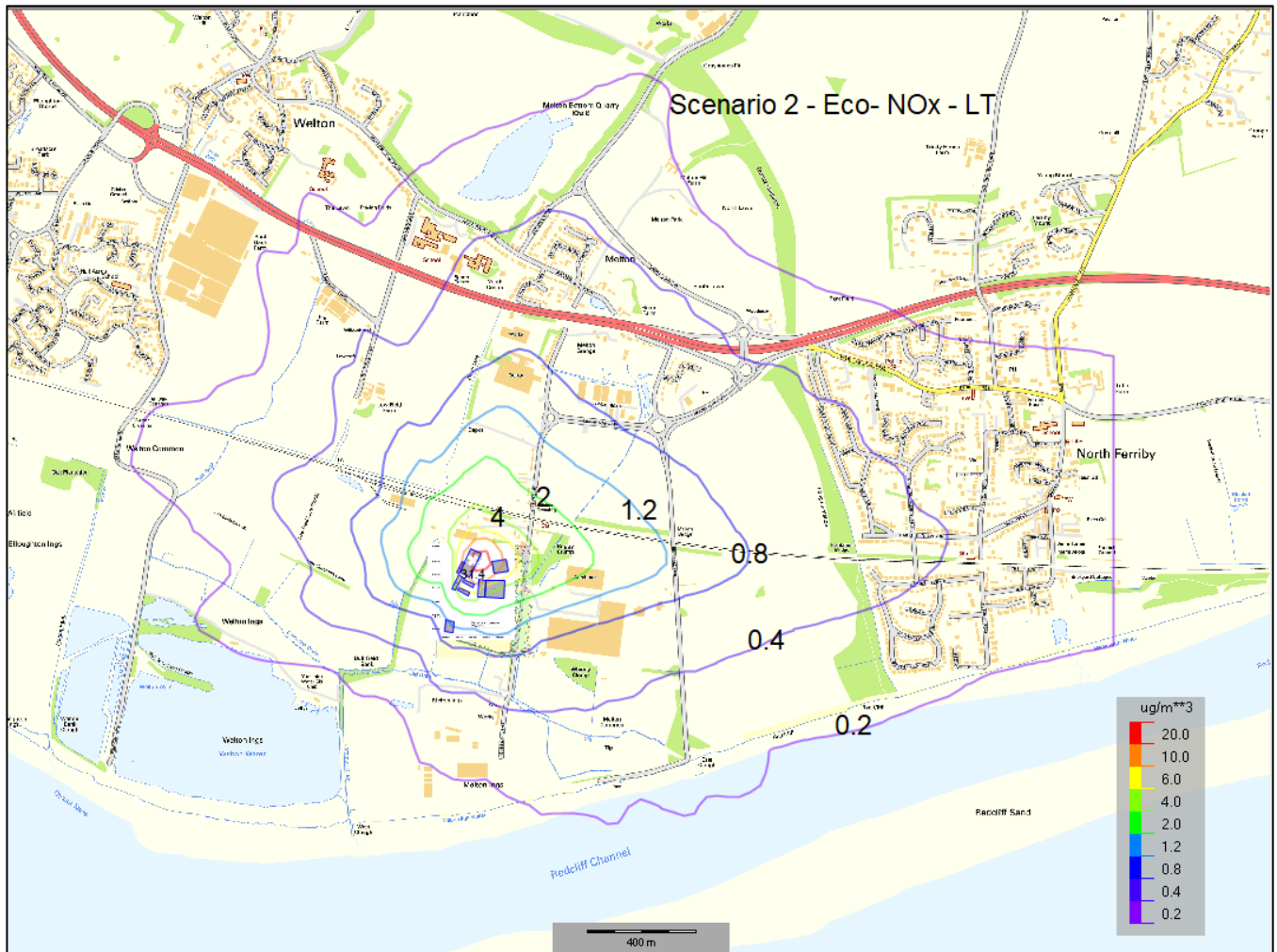
Figure 6-8. Predicted Ground level Long-Term NO x Concentrations (PC) from the Operation of Eco-Power Boilers (2017 Met Data) – Scenario 2
