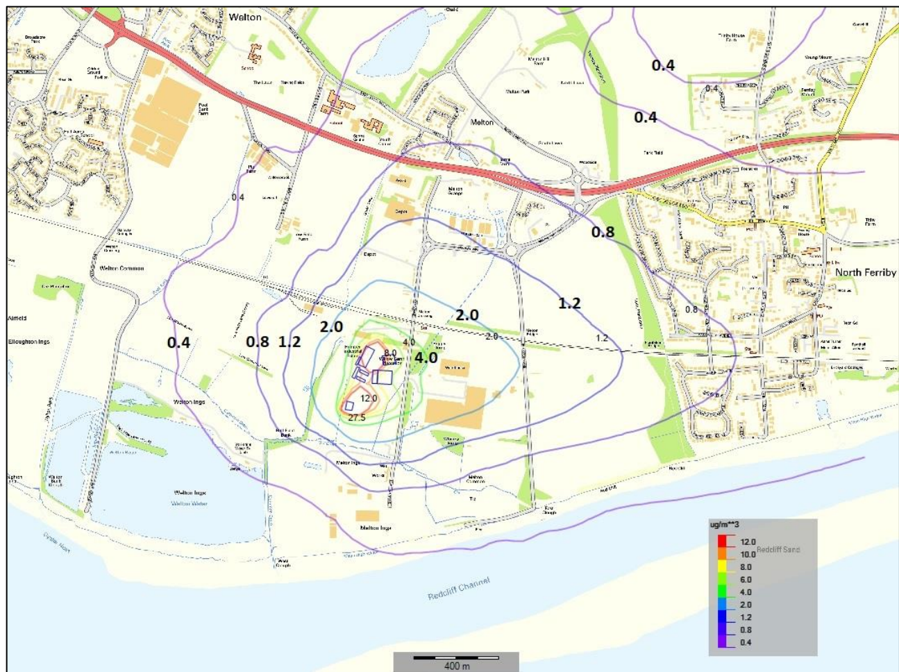
Figure 8-1 Predicted Long-Term NO 2 Concentrations (PC) from the Cumulative Assessment – Including Emissions from Eco-Power Boilers, Transwaste Kalvis Boilers and ERF (2017 Met Data)
