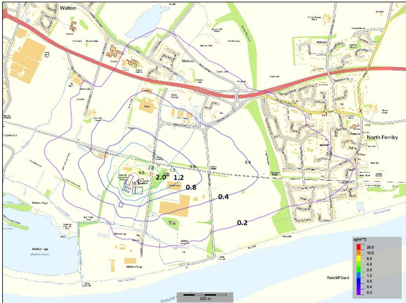
Figure 6-1. Predicted Ground level Long-Term NO 2 Concentrations (PC) from the Operation of Eco-Power Boilers (2017 Met Data) – Scenario 1
