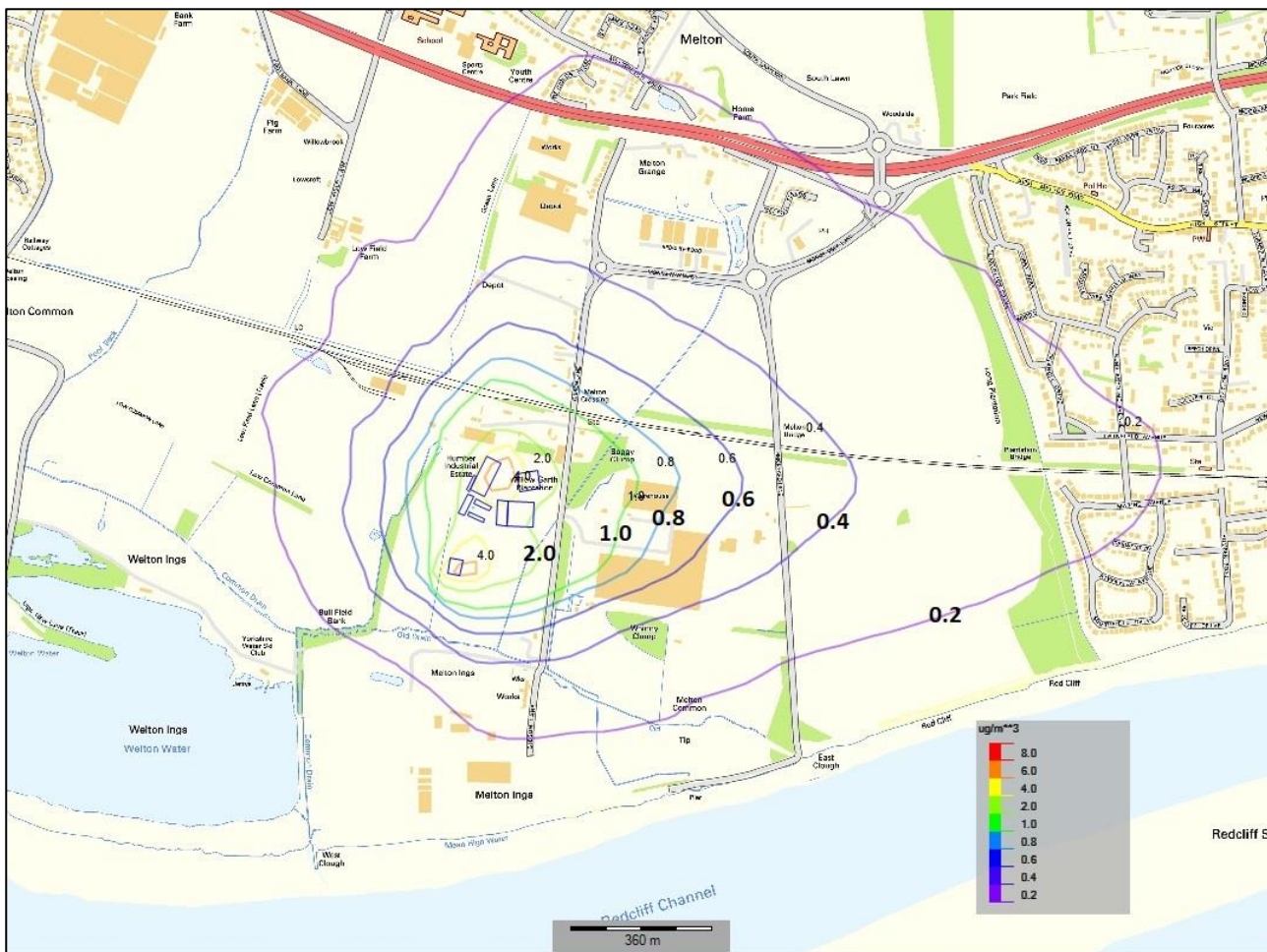
Figure 8-5 Predicted Long-Term PM 10 Concentrations (PC) from the Cumulative Assessment – Including Emissions from Eco-Power Boilers, Transwaste Kalvis Boilers and ERF (2017 Met Data)
