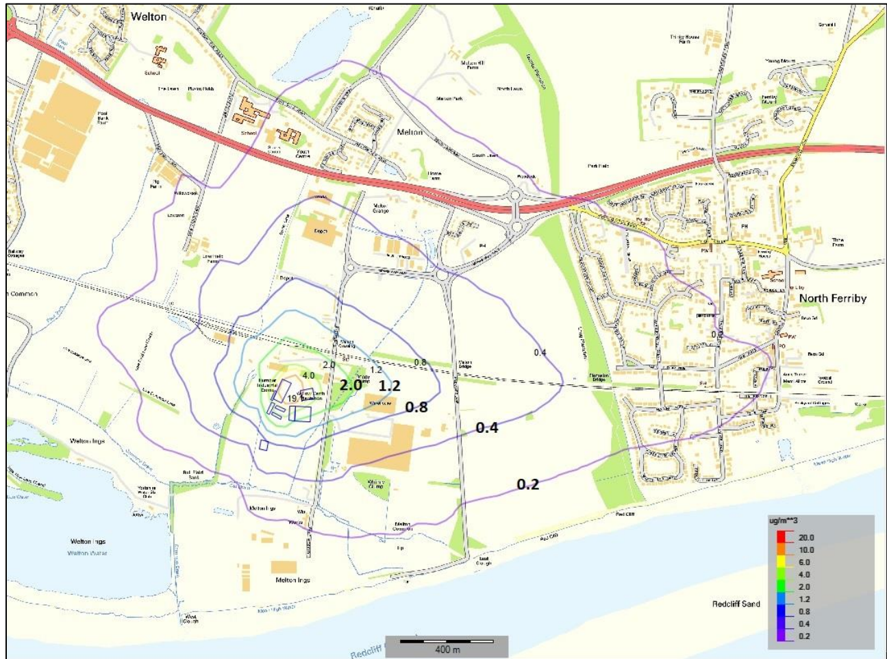
Figure 6-2. Predicted Ground Level Short-Term NO 2 Concentrations (PC, 1-Hour Mean, 99.79 th Percentile) from the Operation of Eco-Power Boilers (2018 Met Data) – Scenario 1
