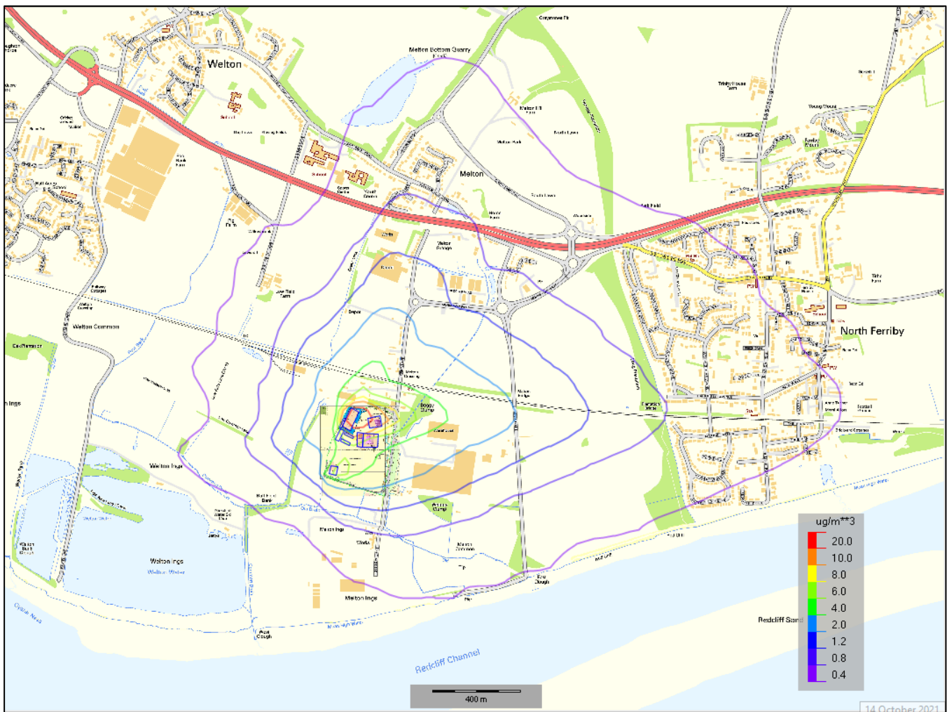
Figure 8-5. Predicted Long-Term PM 10 Concentrations (PC) from the Cumulative Assessment – Including Emissions from Eco-Power Emissions, Transwaste Kalvis Boilers and ERF (2017 Met Data)
