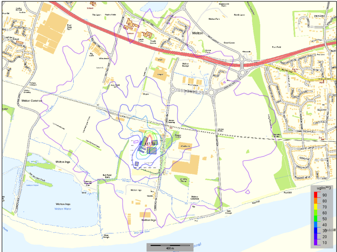
Figure 6-8. Predicted Ground Level Short-Term NO 2 Concentrations (PC, 1-Hour Mean, 99.79 th Percentile) from the Operation of Eco-Power Boilers (2018 Met Data) – Scenario 2
