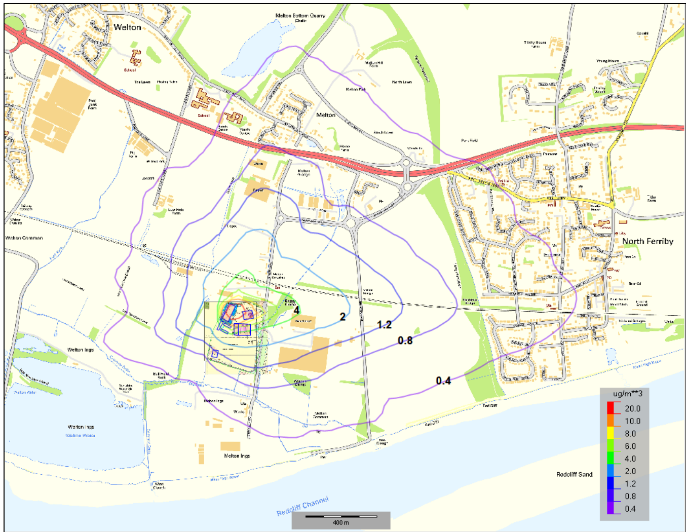
Figure 6-6. Predicted Long-Term PM 10 Concentrations (PC) from the Operation of Eco-Power Boilers (2017 Met Data) (Biomass Boilers + Drying Floor + Cooling Pellets + Dust Extraction System)
