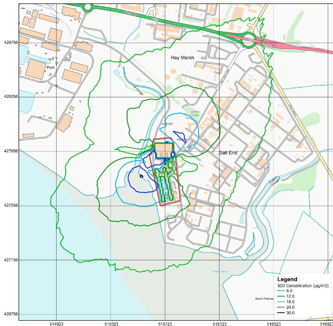
Figure A.2 – 99.73 rd Percentile 1-Hour Mean SO 2 Process Contribution Isopleth (µg/m 3 ) for 2021
