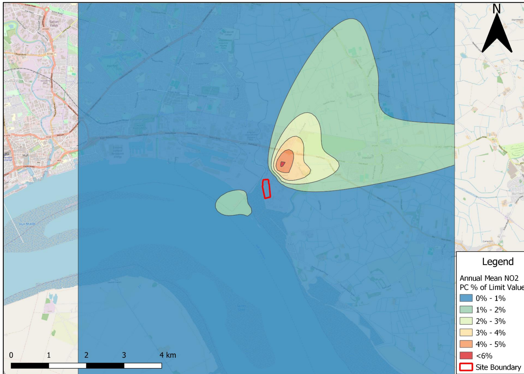
Figure B.2 2020 Annual Mean NO 2 Process Contribution as Percentage of the Limit Value (Limit Value 40 µg/m 3 ) – Proposed
