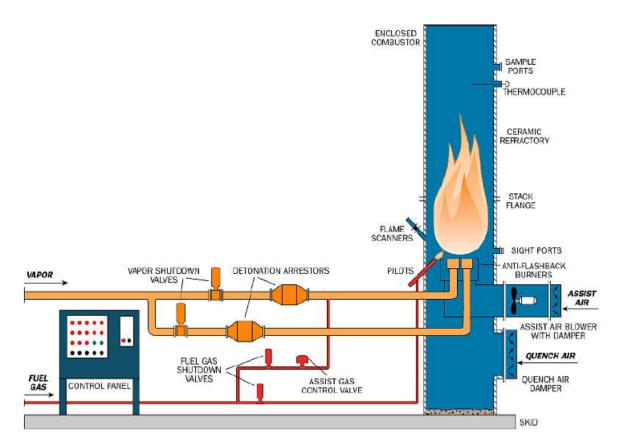
There are two (2) burner stages in the stack. The first stage has one (1) 6" anti-flashback burner. The second stage has two (2) 6" anti-flashback burners.
