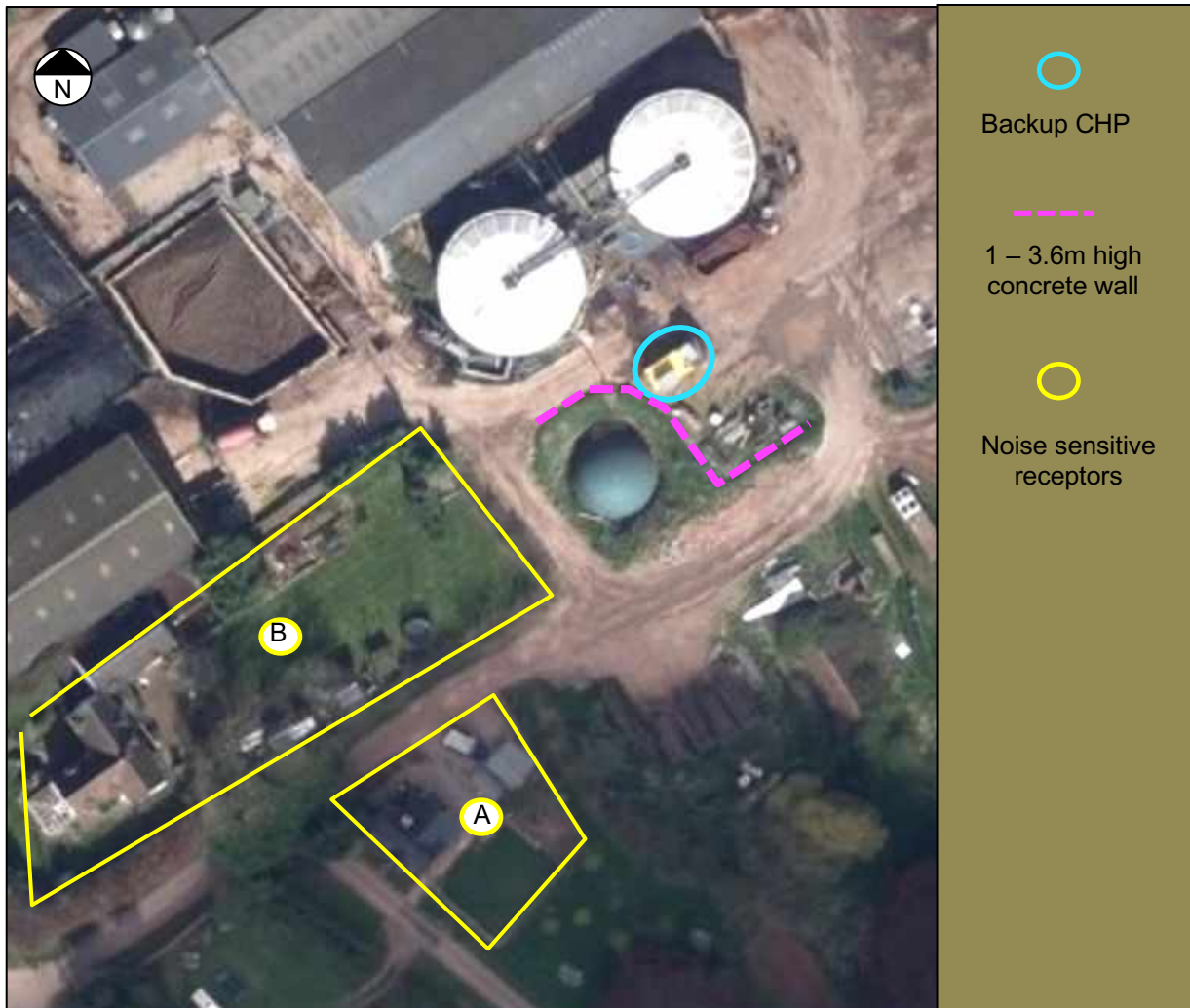
Figure 1. Aerial view (source: bing.com) showing location of backup CHP and nearest noise sensitive receptors
