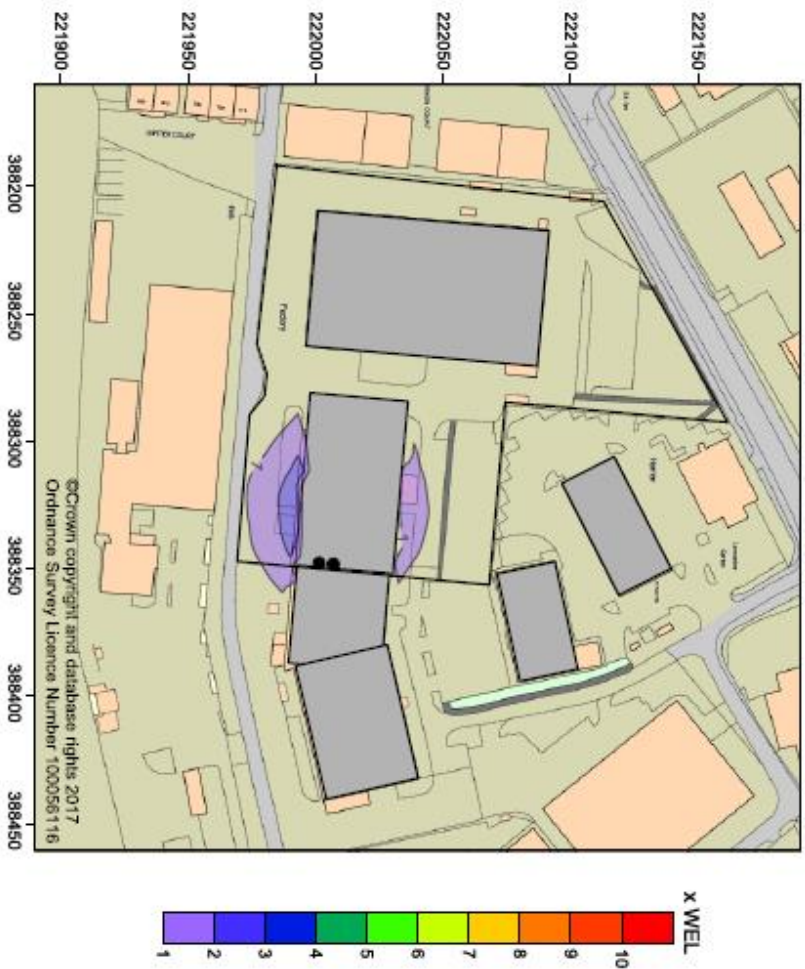
Figure A.11 Scenario 3B - Predicted concentrations of hydrogen cyanide (maximum 15 minutes mean - WEL) at 1.5 m
