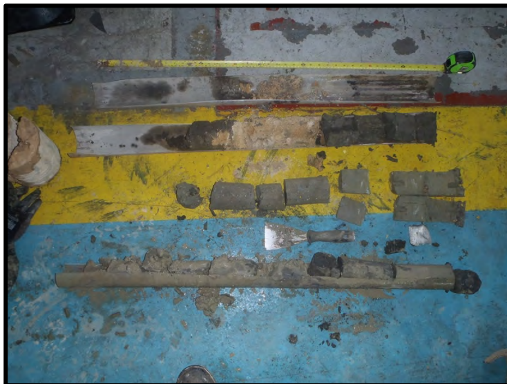
Borehole Core: 0.0-3.0m
