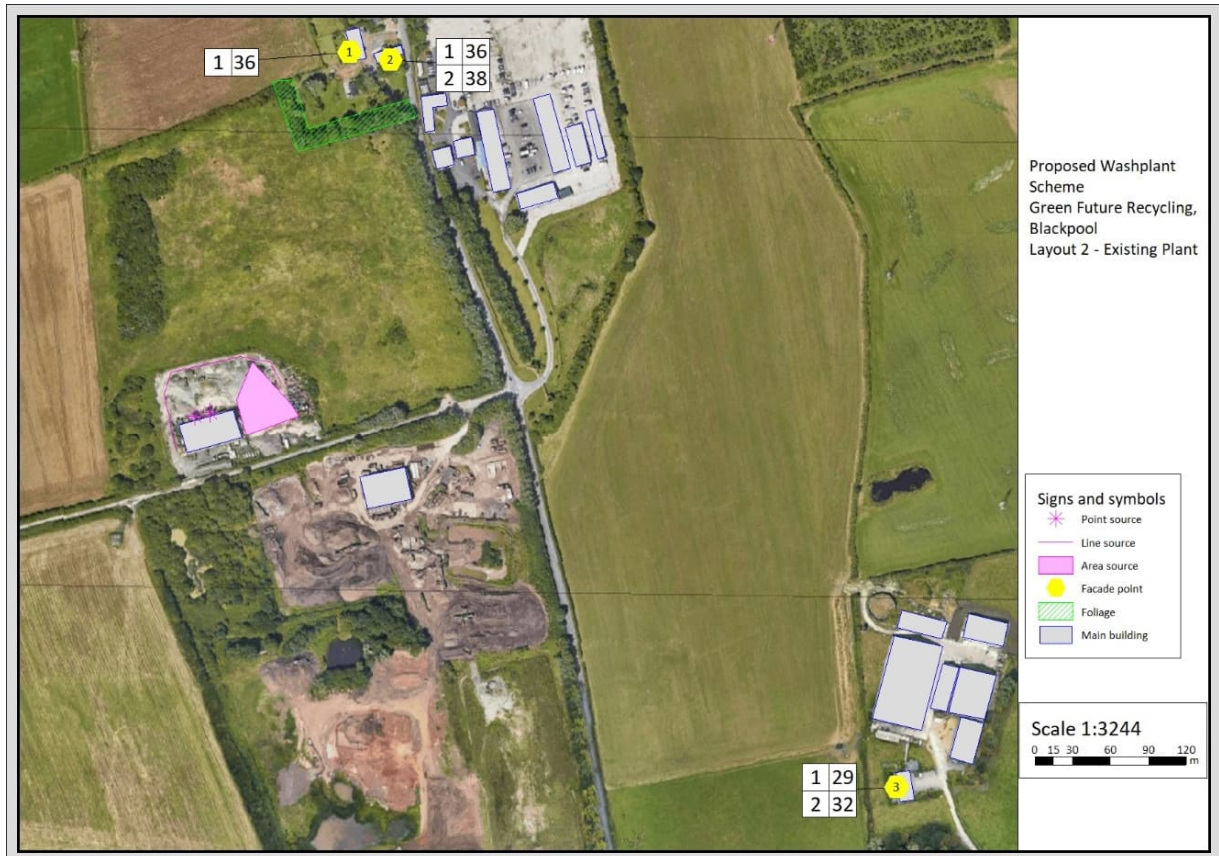
Figure 2 - SoundPlan model – Calculated noise levels at receivers with pre-existing plant on site
