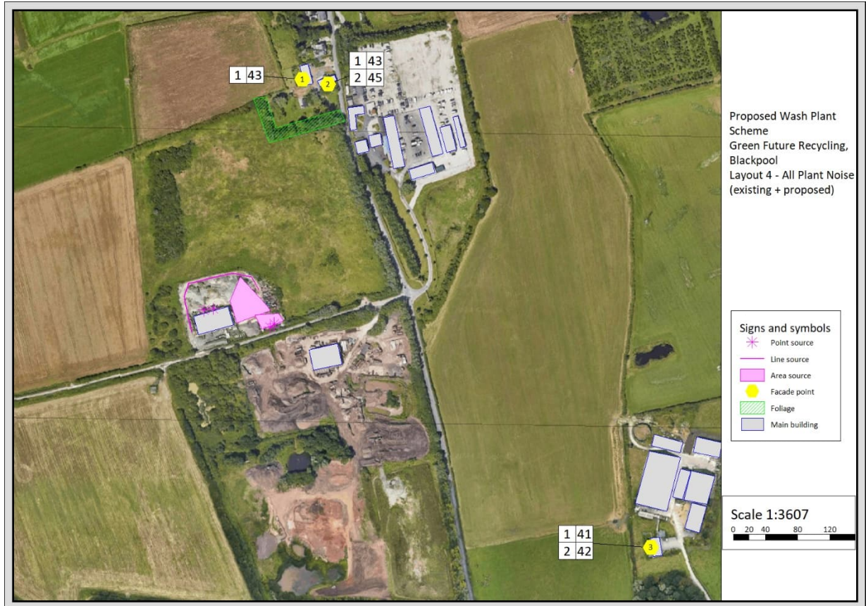
Figure 4 – SoundPlan model – Calculated noise levels at receivers with existing and proposed plant on site
