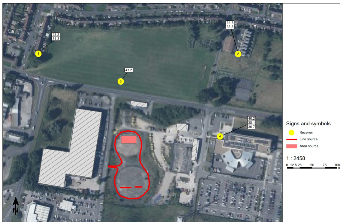
Figure 17 – Sound levels due to emergency access of lorries only to the site
