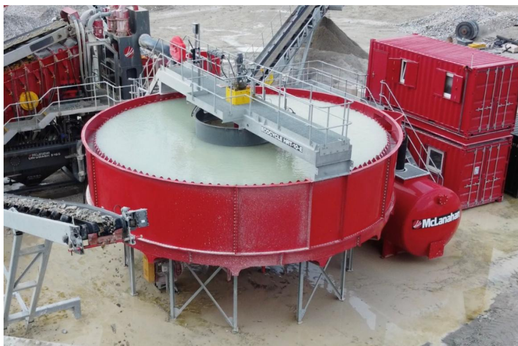
Figure 1. Photograph of McLanahan Thickener
