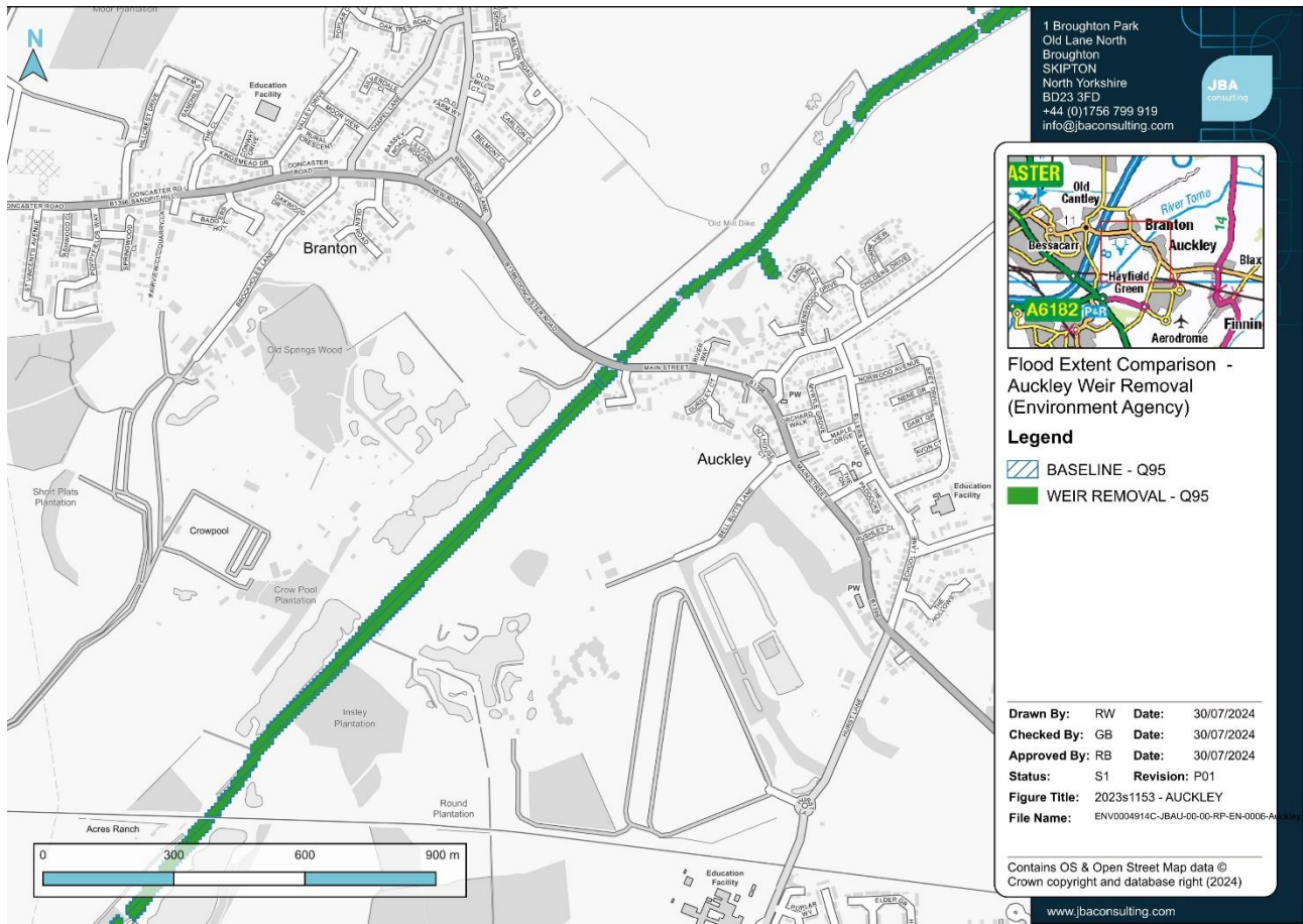
Fig. A-6: Q95 low flow event flood extent - baseline versus proposed weir removal
