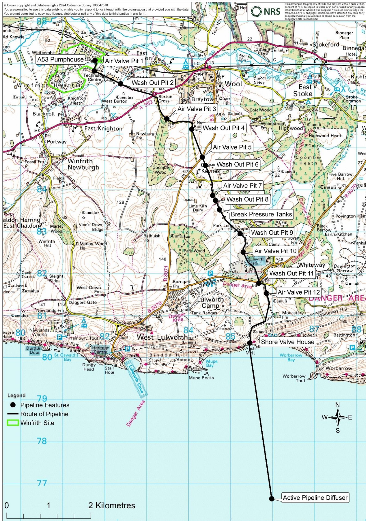
Figure 2.1: Ordnance Survey map showing the Winfrith nuclear licensed site (green outline) and the route of the Sea Discharge Pipeline (black line) [35]. The site and the route of the Pipeline form the area covered by the Winfrith RSR permit [7].
