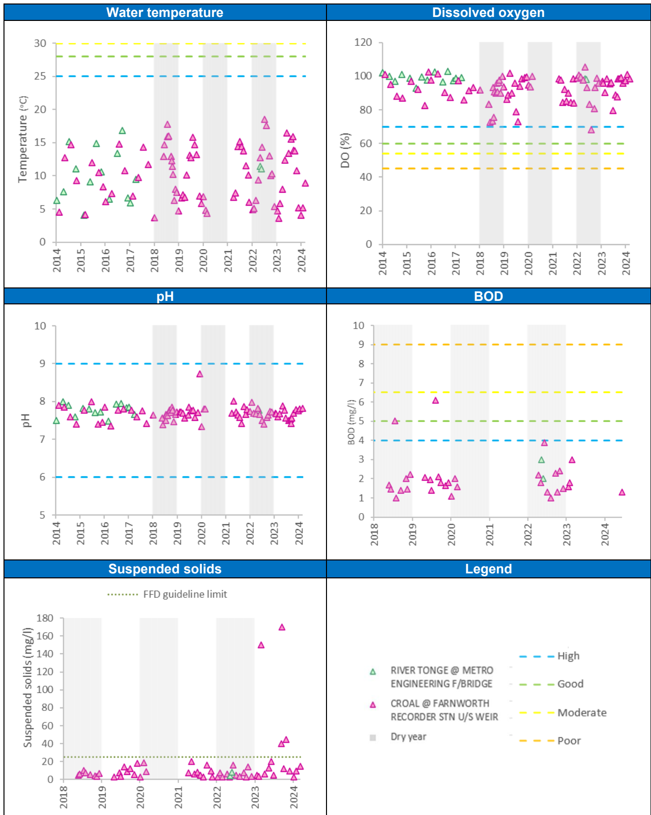
Figure A2-27 Physico-chemical parameters recorded at EA monitoring locations within the Rivers Tonge and Croal (including Blackshaw Brook) water bodies (GB112069064530 and GB112069064550)
