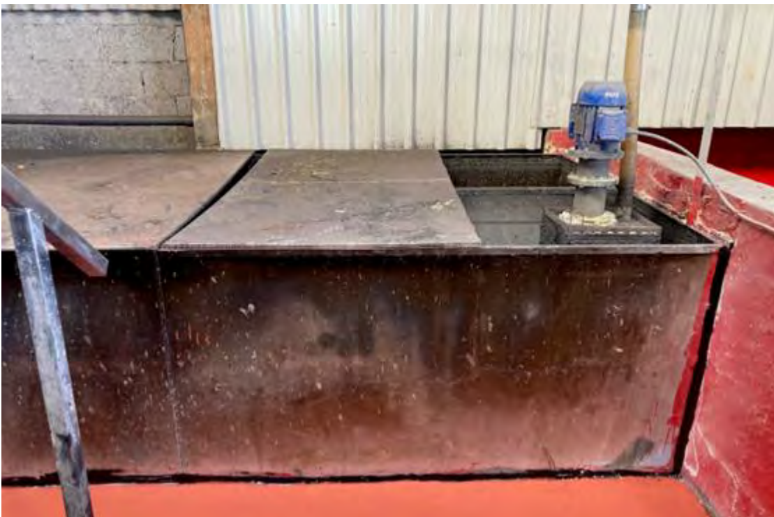
Photo 3: Lead sludge tank. This will not be used in the future process as battery breaking will become automated
