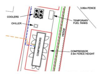
The corrections for equipment size which would apply to the compressor enclosure would be 23dB and for the smaller cooler unit, 19dB. The sound power level of the compressor enclosure would therefore be LwA 87dB and the cooler LwA 76dB.
