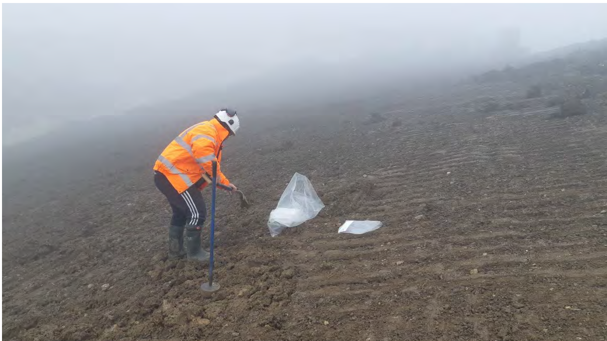
Extraction of clay cores using core cutter on west clay lined area of Phase 1 north batter
