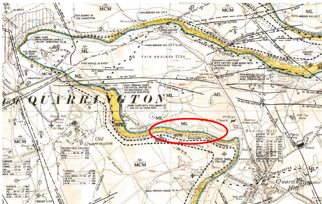
Figure 2 – Local Geology. Extract from BGS Sheet NZ33NW. East-west ridge formed by Permian strata. Marl Slate (blue) and Yellow Sands (Yellow) outcropping on flanks of ridge. Site circled in red.
