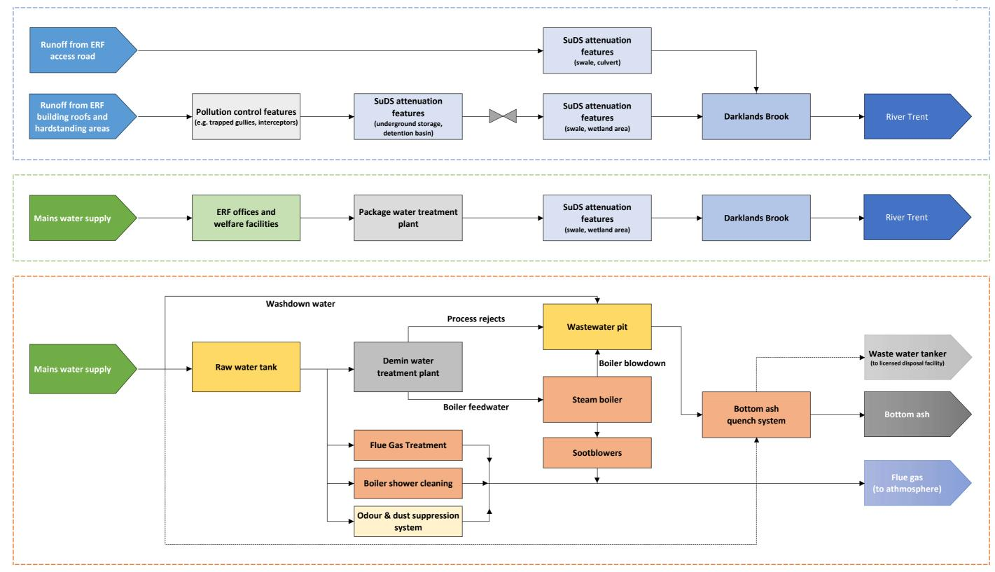
S4081-0100-0005RO SERF Indicative Water Flow Diagram Rev. 0
