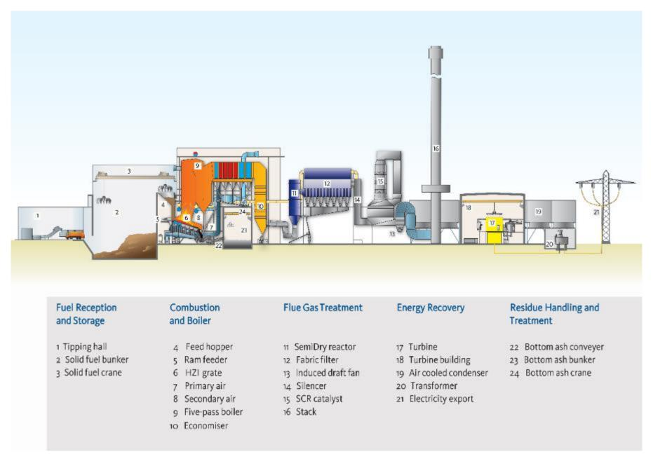
Figure 1– Indicative Schematic of the ERF
