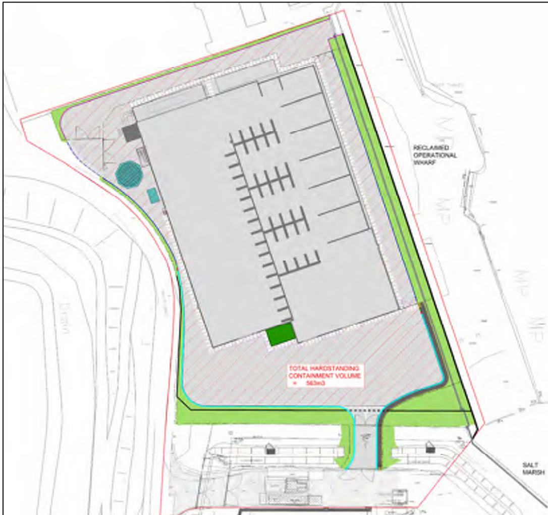
Figure 4.3 Area of proposed secondary spent fire water containment on hardstanding apron
