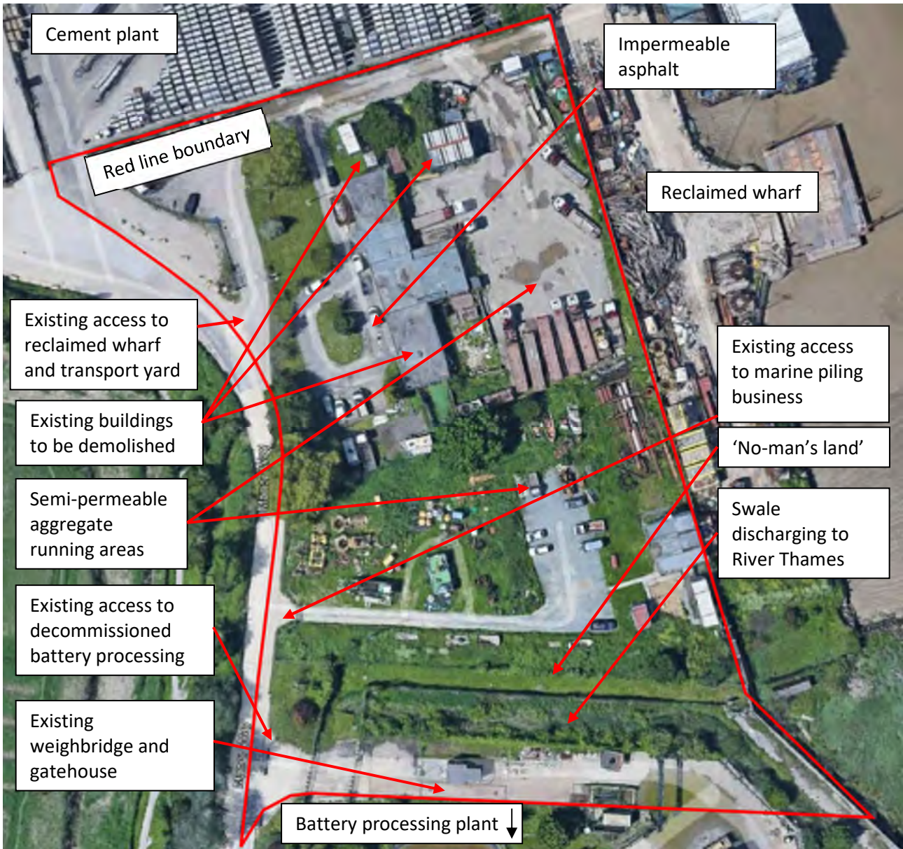
Figure 1.1 Proposed E-Scrap facility site location
