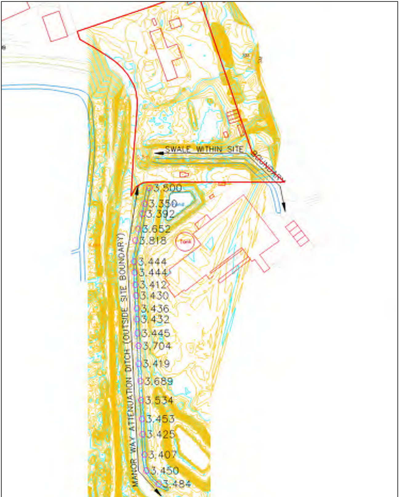
Figure 2.1 Existing Manor way ditch bed levels (mAOD). Taken from EA LiDAR data.
