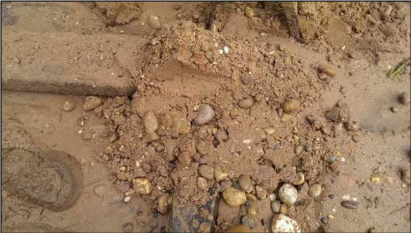
Photograph 38: BH3 - Gravelly sand from between 12.4m and 14.2m.
