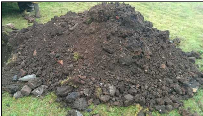
Photograph 27: TP8 - Blackish sand arisings from between 1.9m and 3.9m with quartz and quartzite gravel, brick and concrete together with glass bottles, a bike wheel and plastic.
