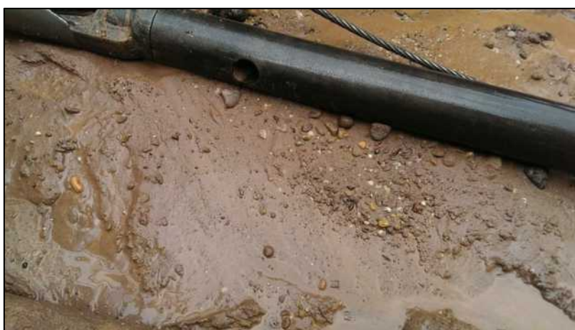
Photograph 41: BH4 - Silty gravelly sands between 11.2m and 14.2m
