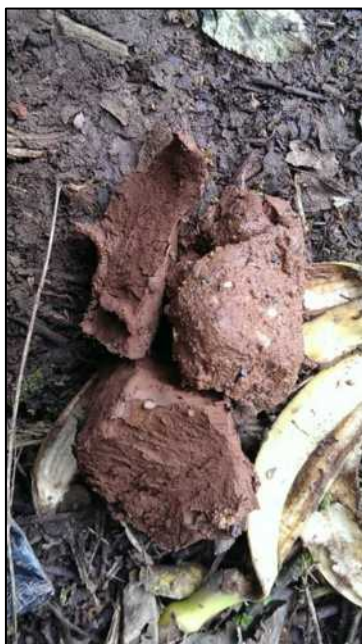
Photograph 42: Reddish brown clay at the base of the borehole, overlying a cobble at 14.5m.
