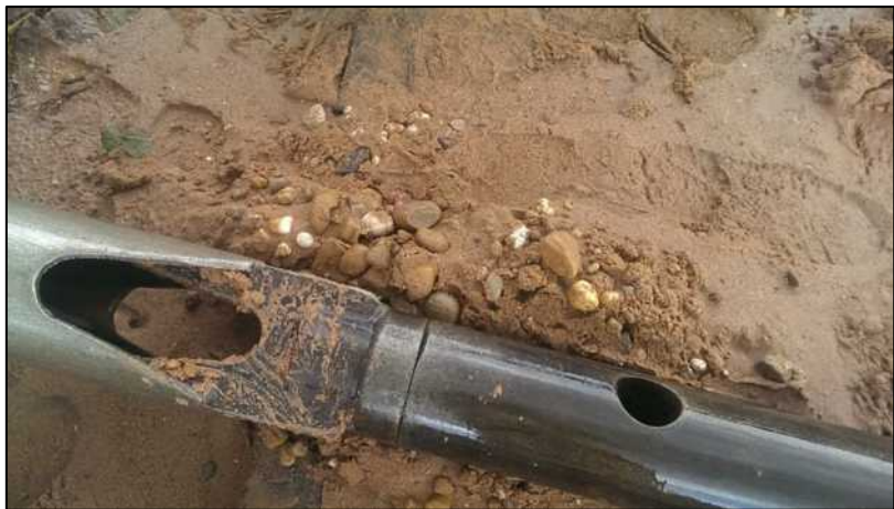
Photograph 34: BH2 - Sands and gravels encountered between 10.3m to 13.5m.
