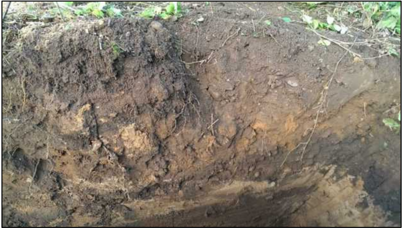
Photograph 1: TP1 - The upper 0.7m of Made Ground.
