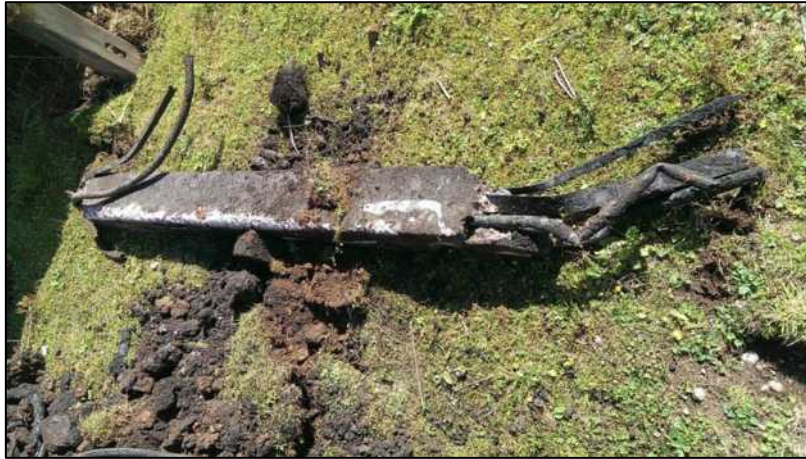
Photograph 23: TP6 - One of two 1.5m concrete cable piles found within the trial pit between 1.0m and 3.0m.
