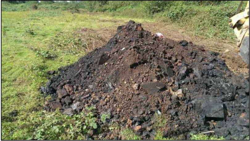
Photograph 12: TP4 - Odorous blackish sand from 1.2m with gravel, concrete, bricks, metal, wood and plastic.
