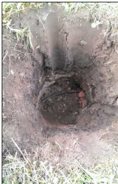
Photograph 35: BH3 - Brick and metal at 0.5m within the hand pit.
