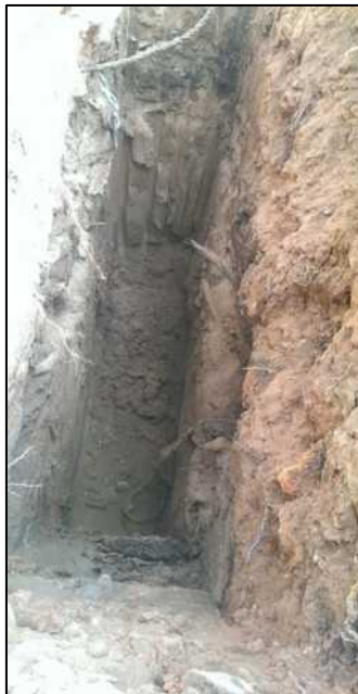
Photograph 14: TP4 - rope, wood and rubble within the sidewalls. Slightly unstable in the sand at 1.1m,.
