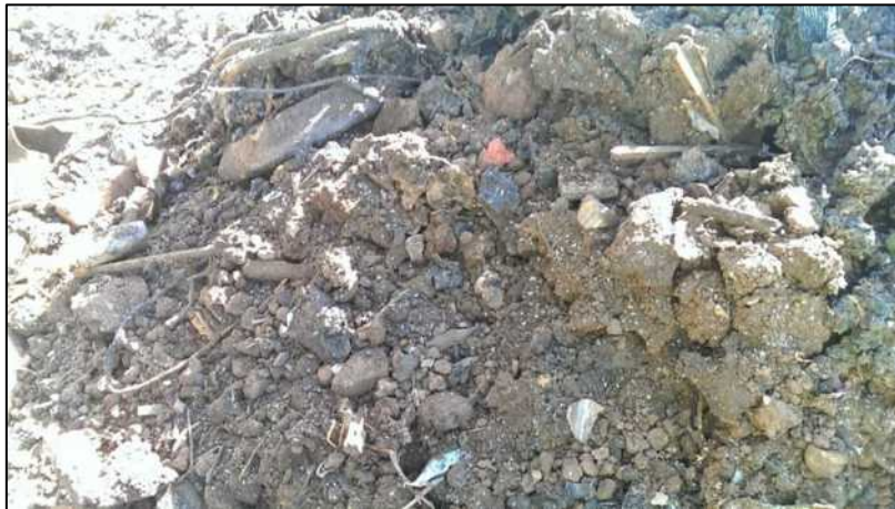
Photograph 5: TP2 - Close up of rubble, plastic and wood in the clay arisings.
