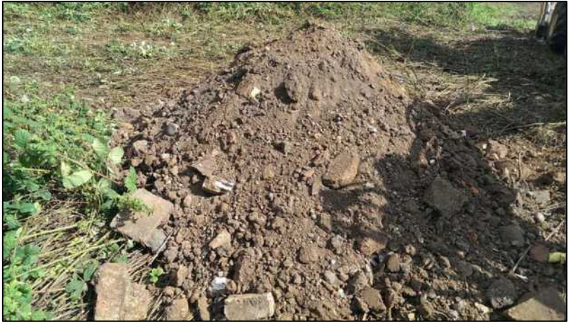
Photograph 10: TP4 - Orangey brown sand of the upper 1.2m material with rubble of quartz and quartzite gravel, brick and concrete.
