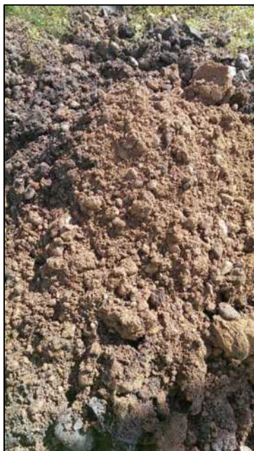
Photograph 30: BH1 - Orangey brown clayey sand encountered between 5.4m and 6.8m.
