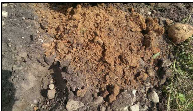
Photograph 36: BH3 - Orangey brown sand with brick fragments from between 1.3m and 4.2m.
