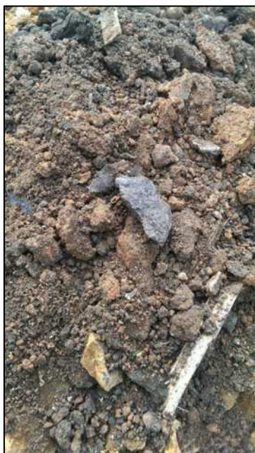
Photograph 29: BH1 - Asphalt in the Made Ground encountered between 0.7m and 4.8m
