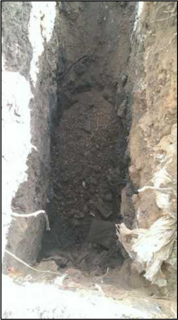
Photograph 11: TP4 - Base of trial pit and small collapse from the rubble in the blackish sand at 1.2m. Plastic bag at 0.5m.
