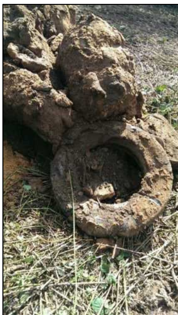
Photograph 16: TP4 - One of two inner tyre tubes recovered from 3.1m within the sandy clay.
