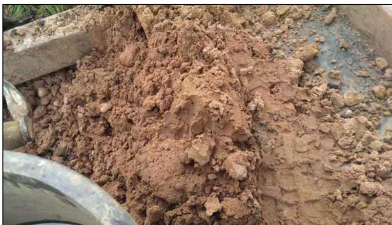
Photograph 31: BH1 - Silty slightly gravelly sand of the natural ground, at 6.8m.
