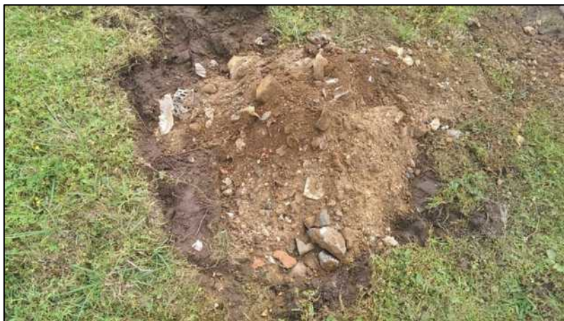
Photograph 28: BH1 - Light orangey brown gravelly sand of the upper 0.7m excavated from the 1m hand pit.
