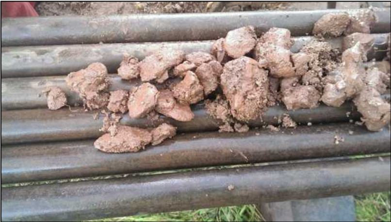
Photograph 39: BH3 - Clayey sandy gravels at the base of the borehole, interpreted as Mercia Mudstone
