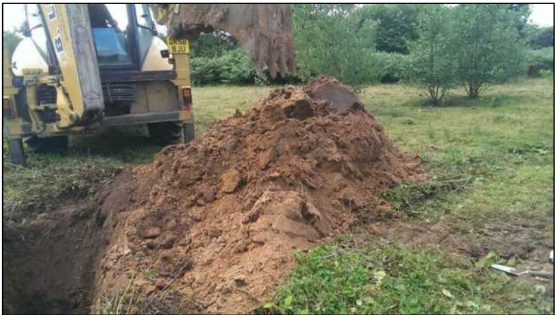
Photograph 2: TP1 - Light orangey brown silty sand arisings from between 0.7m and 3.6m
