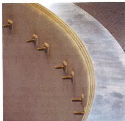
Typical Chamber Shunt Bolts
