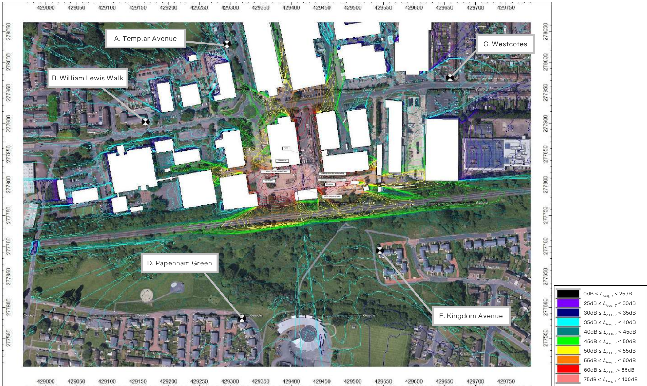
Figure D1: Predicted daytime Specific Sound Level, L_{Aeq,1hour} at 4 metres grid height – existing plant (Google 2026)
