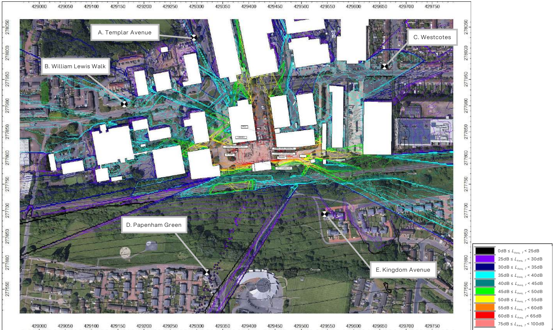
Figure D2: Predicted daytime Specific Sound Level, L_{Aeq,1hour} at 4 metres grid height – proposed new plant (Google 2026)
