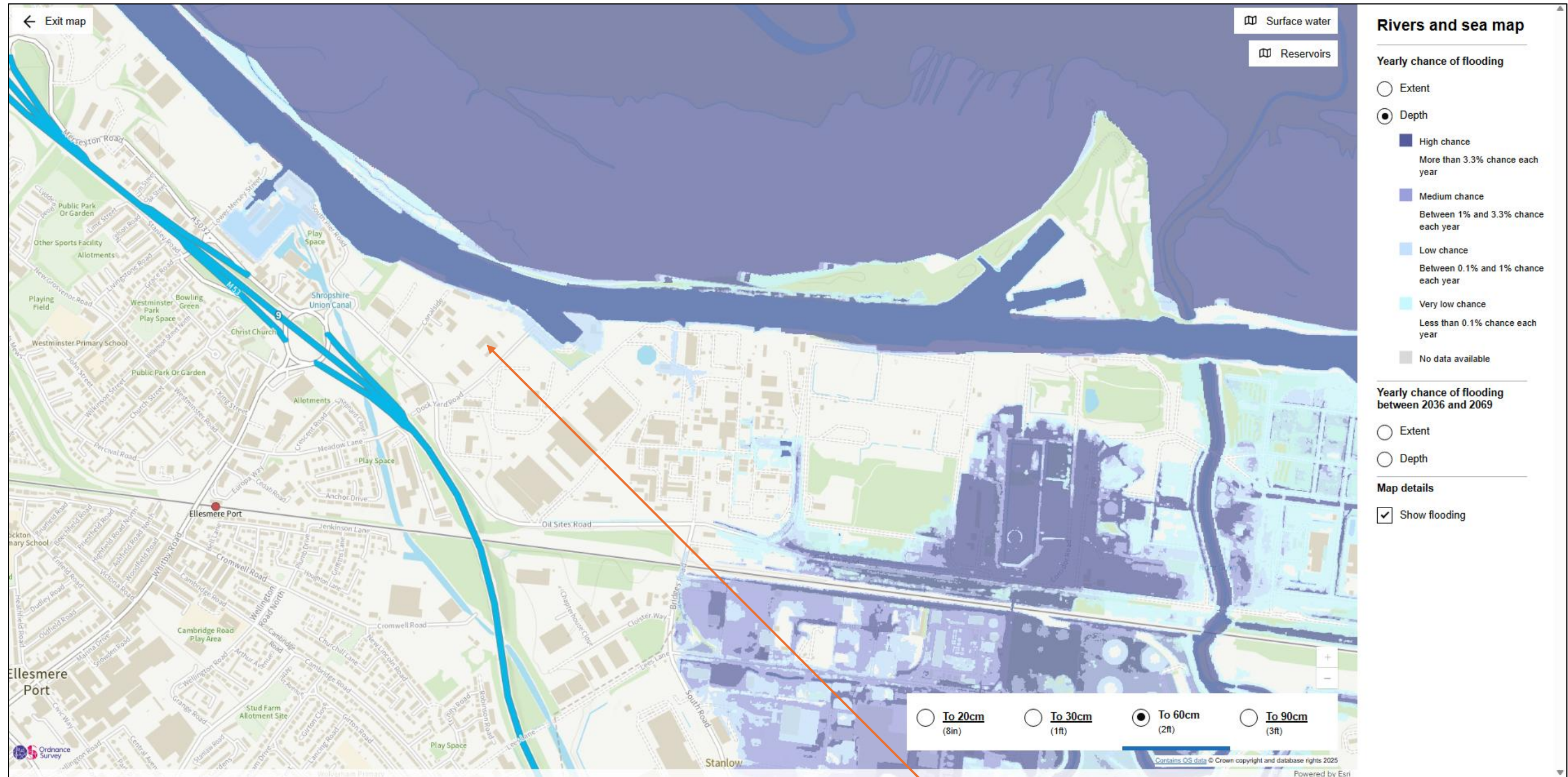
Figure 8 Shows the risk of flood from rivers and sea showing the dept of flooding between 2036 and 2069 to 60cm for the site
