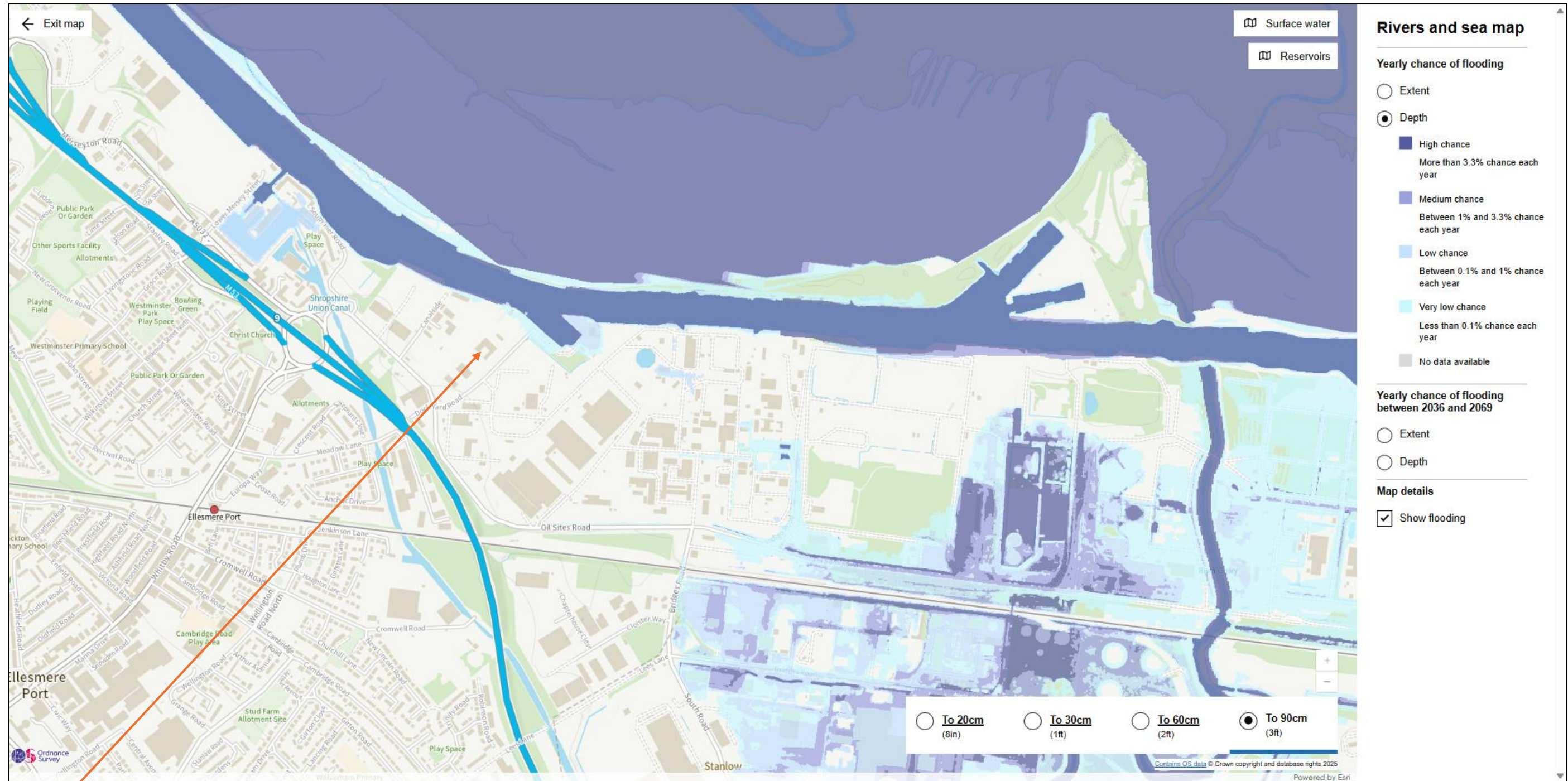
Figure 9 Shows the risk of flood from rivers and sea showing the dept of flooding between 2036 and 2069 to 90cm for the site
