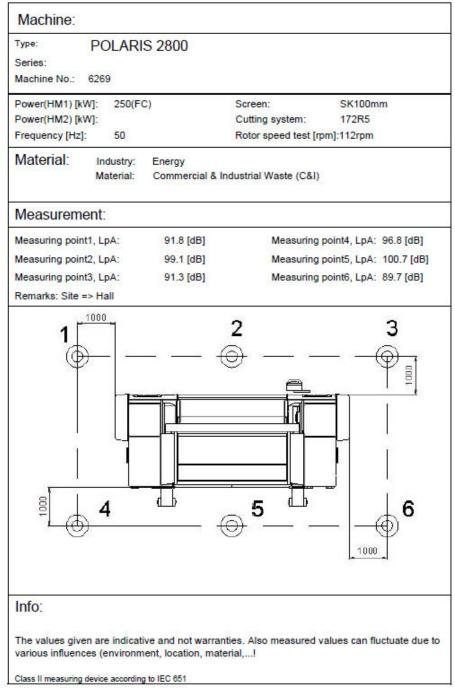
Figure D1: Polaris Shredder Manufacturer's Noise Data
