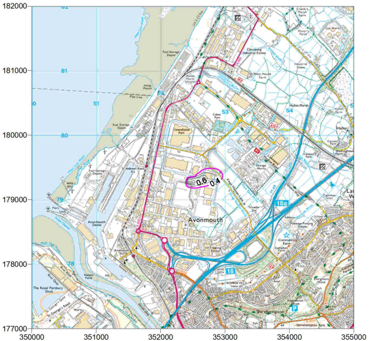
Figure 8 Annual Average Process Contribution of NO x as NO 2 (µg m -3 ); 2019 Meteorological Conditions. Magenta Isopleth Denotes the Point of Insignificance (1 % of the Objective Value)
