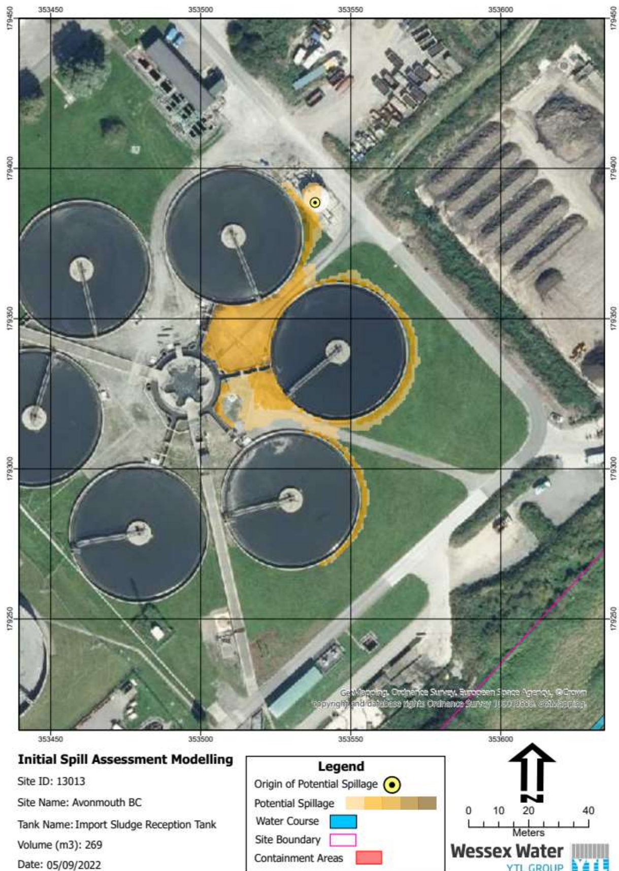
Figure 8.7: Spill Assessment for Imported Sludge Reception Tank
