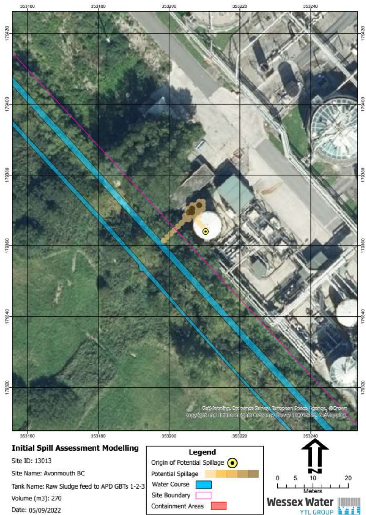
Figure 8.15: Spill assessment model for APD GBTs 1, 2 and 3 Feed Tank
