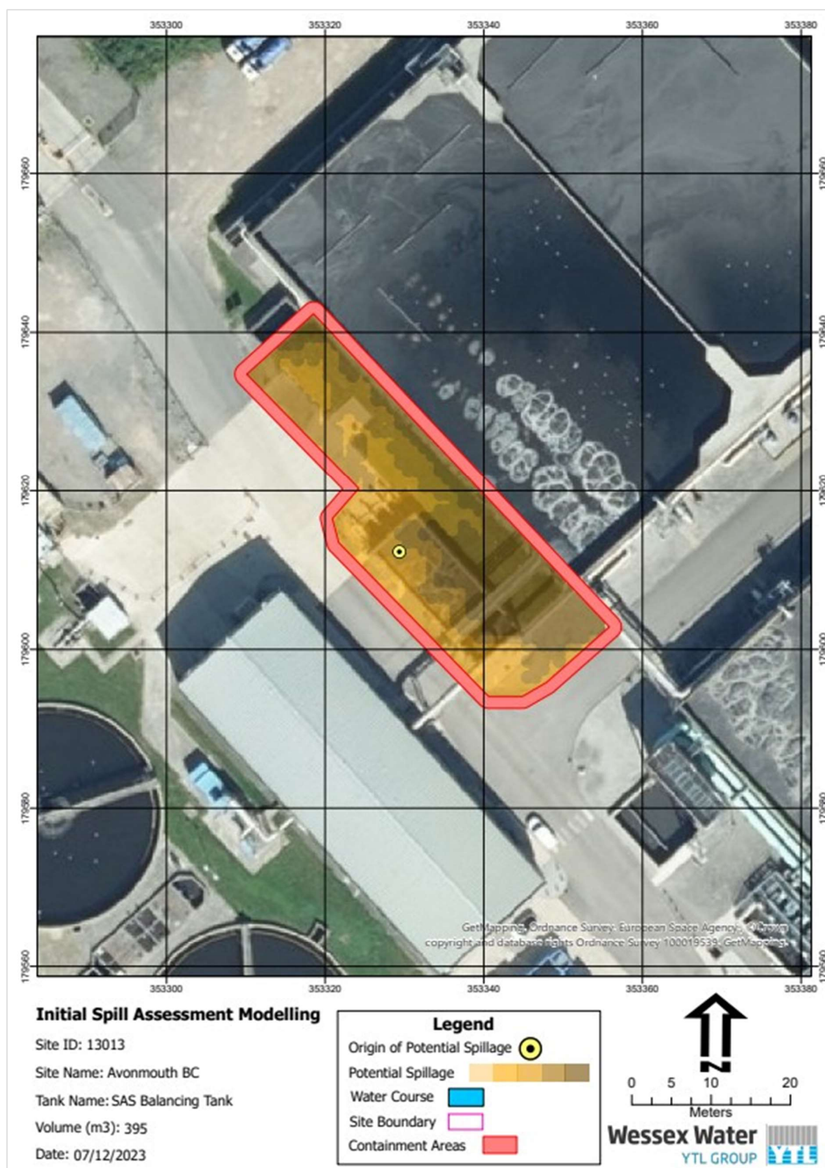
Figure 9.3: SAS Balancing Tank Containment Proposal Spill model.
