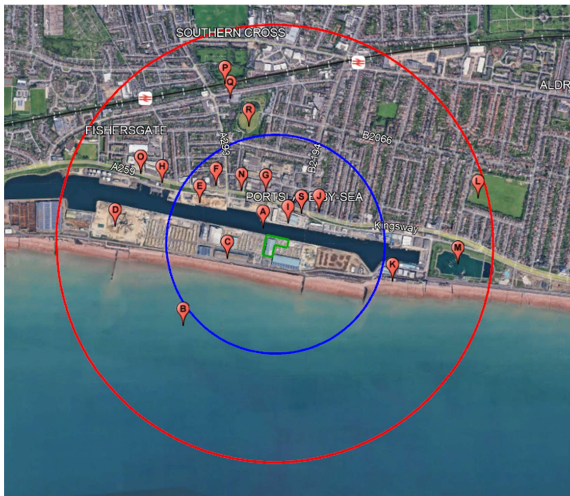
Figure 2 - Site Setting and Receptors (The permitted site is shown with a green boundary). Blue shows 500m radius from centre point of site. The red line shows 1km radius from the centre of the site.
