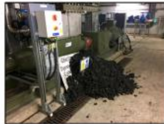
Figure 14: Ex sign & spillage from silo.
