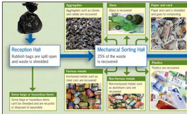
Figure 5: How an MBT plant works Source: Anon
