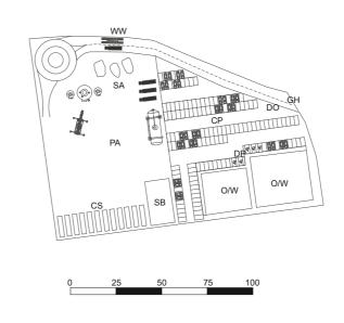
Proposed general arrangements for temporary construction compounds (TCCs). Only one TCC to be implemented.
