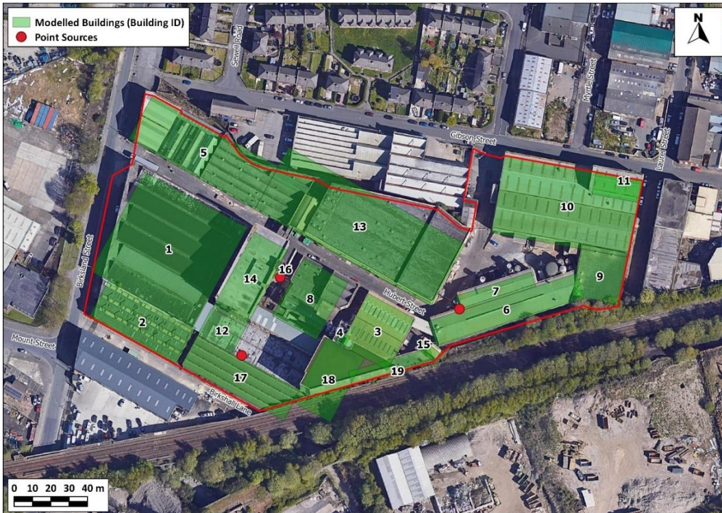
Figure 10: Buildings Included in the Model (Green-topped Objects) and Modelled Flues (Red-topped Cylinders)
