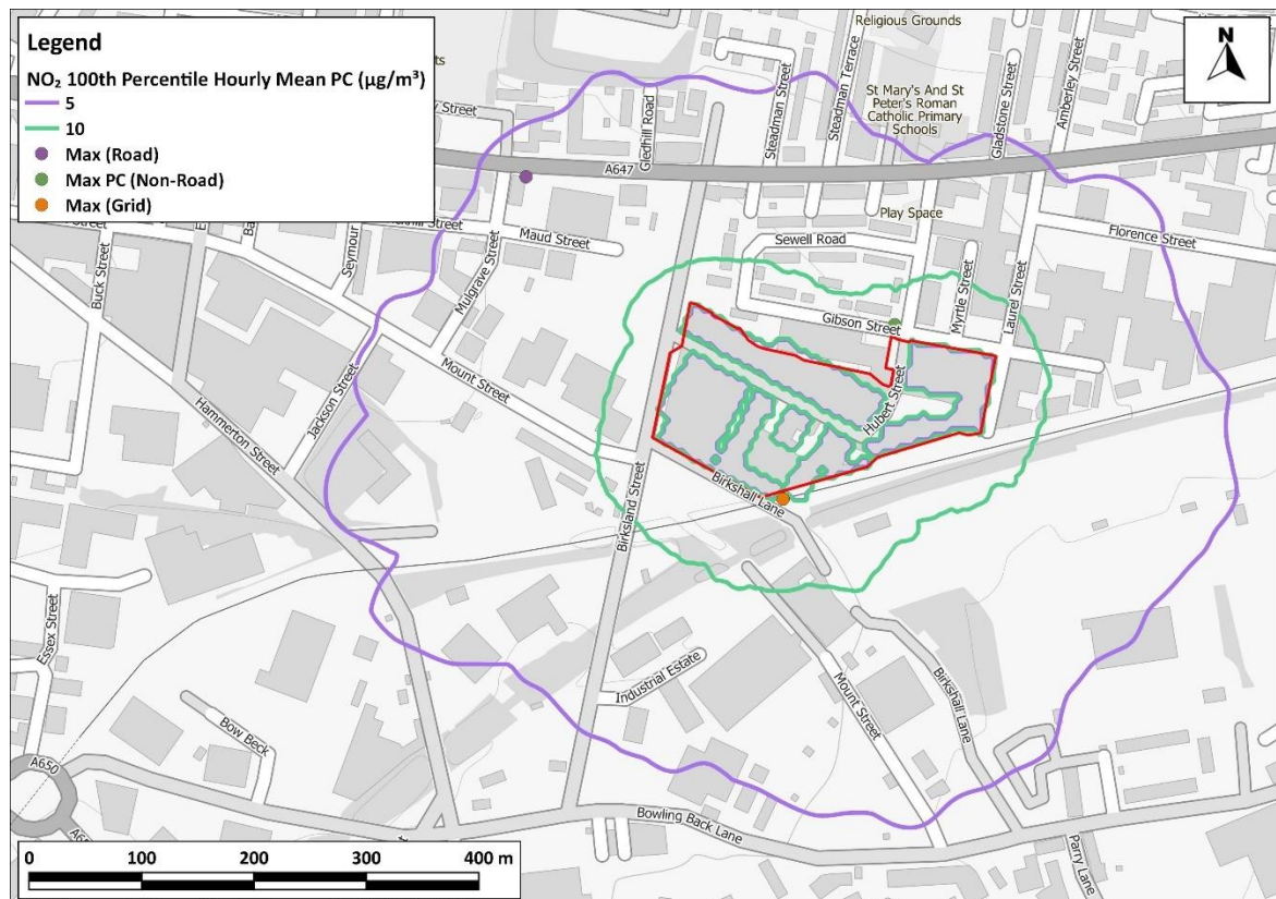
Figure A3.1: Contour Plot of the 100 th Percentile of 1-hour Mean NO 2 PCs
