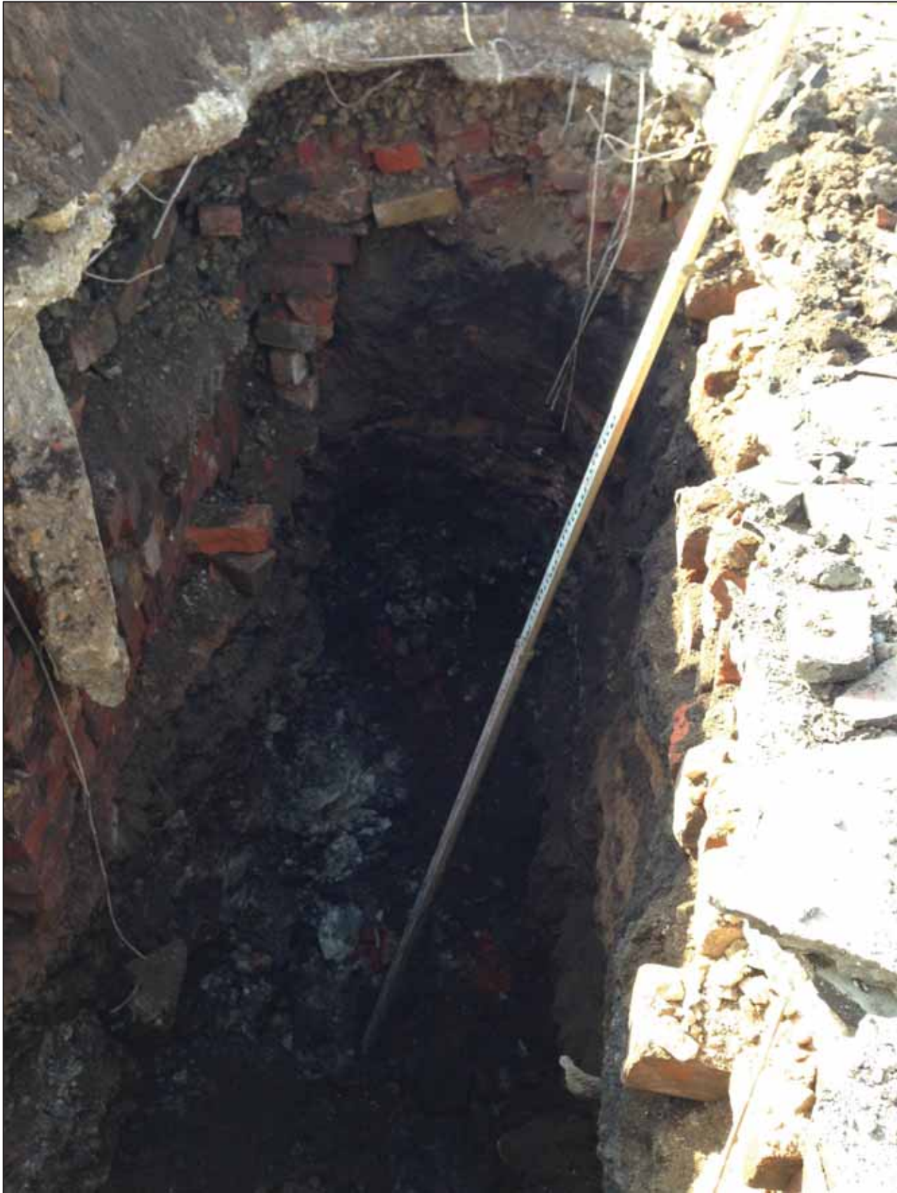
Photograph 8: Trial Pit BH4-TP (Layer of slag at base at approx. 1.80 m bgl )
