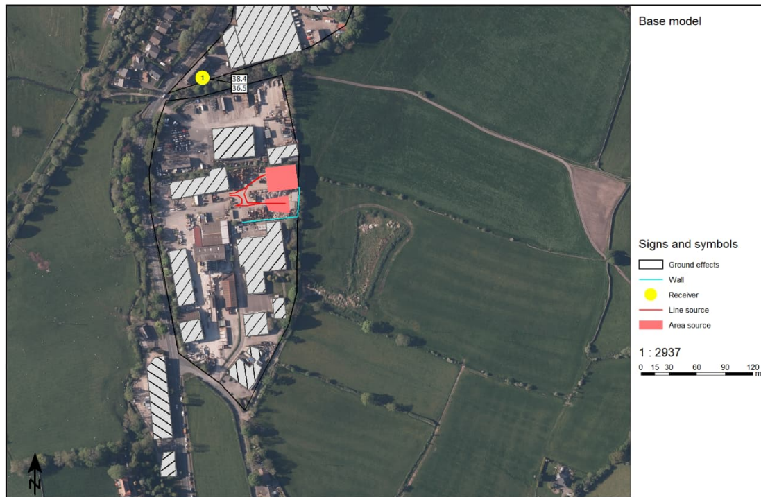
Figure 5 - SoundPlan model - sound propagation to nearest noise sensitive properties with existing permitted waste transfer operations – Tables give sound pressure level for the indicated floor heights
