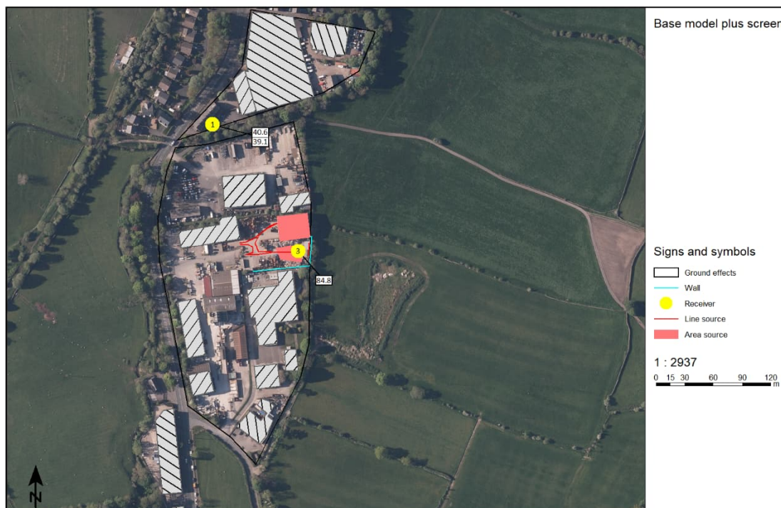
Figure 6 - SoundPlan model - sound propagation to nearest noise sensitive properties with proposed screening plant operational – Tables give sound pressure level for the indicated floor heights
